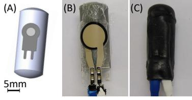
**Fig. 2:** Development of robotic capsule prototype. (A) CAD model (B) Capsule prototype with force sensor glued on the capsule. (C) Capsule prototype with water resistant lamination.
