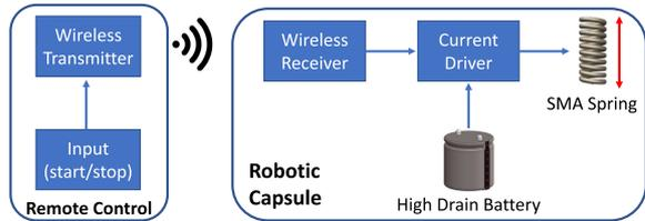
Fig. 6. Actuation mechanism of robotic capsule.
