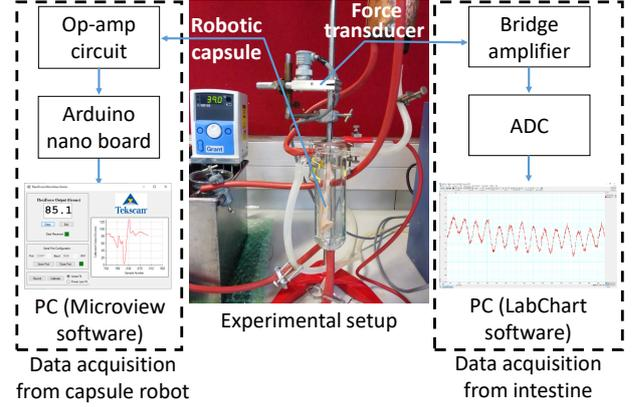
**Fig. 4:** Data acquisition system for peristaltic and axial force measurements. (Left side) data acquisition system of robotic capsule measures the peristaltic forces. (Right side) data acquisition system of in-vitro system measures the axial forces.
