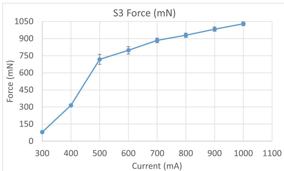
Figure 5.15: Force analysis of two-way SMA spring actuator - variation of forces for Spring 3 (S3)
