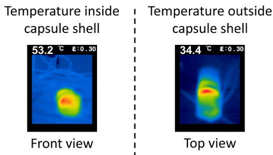
**FIGURE 9.** Temperature profile of robotic capsule at 500 mA current recorded by thermal imaging camera.
