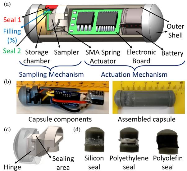
Fig. 1. Standalone robotic capsule for gut sampling. (a) CAD model. (b) Robotic capsule prototype. (c) Hinge mechanism between sampler and storage chamber. (d) Tested sealing materials at the hinge mechanism.
