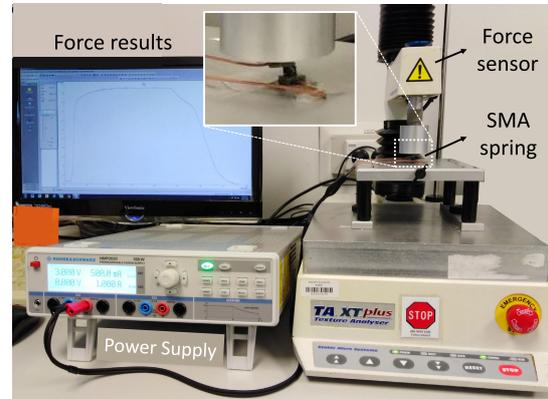
FIGURE 4. Experimental setup for force measurements of SMA spring.
