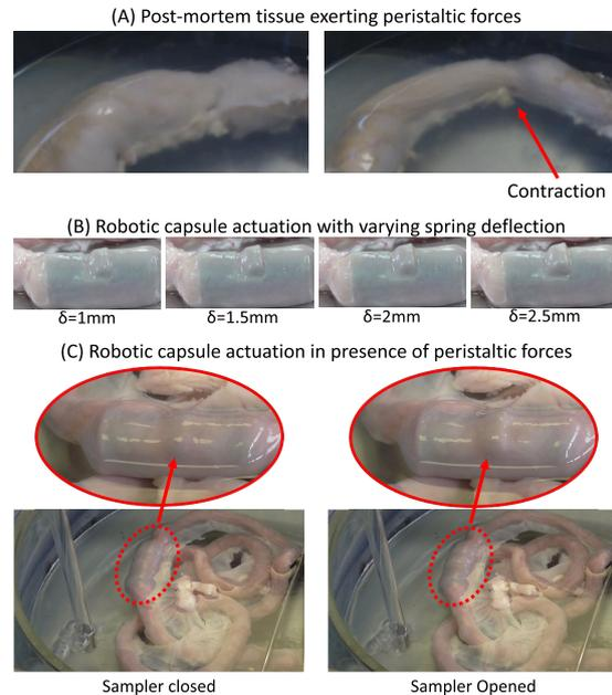
**FIGURE 10.** Sample collection process under in-vitro experimental setup.
