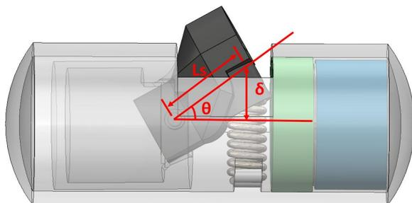
FIGURE 3 Mathematical relation between sampler and actuator
