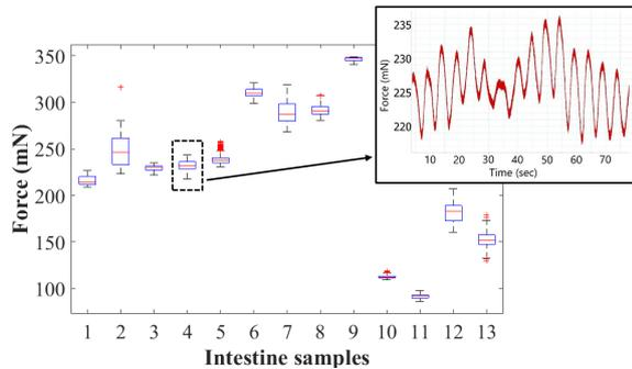
**Fig. 7:** Variations in axial forces generated by 100 mm intestinal tissue samples measured by the axial force transducer. In each sample, top and bottom bars show the range of axial forces, rectangular box indicates first and third quartile, red line shows the median and red plus sign shows the outliers. Window at top right shows a sample of force measurement data, plotted by LabChart software.
