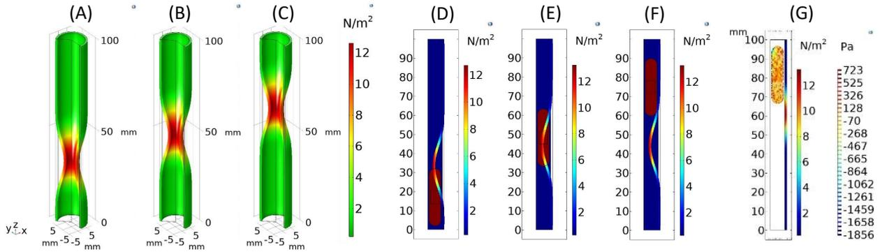
**Fig. 6:** Simulations performed in COMSOL Multiphysics. (A)-(C) 3D view of repetitive peristaltic wave of 7 seconds/cycle generated across the 100 mm intestine (A)  $t = 0.5$  sec, (B)  $t = 3.5$  sec, (C)  $t = 6.5$  sec. (D)-(F) 2D-axisymmetric view of robotic capsule interacting with the intestine due to the repetitive peristaltic movement (D)  $t = 0.5$  sec, (E)  $t = 22$  sec, (F)  $t = 32$  sec. (G) Pressure experienced by the robotic capsule due to radial contraction of the intestine.
