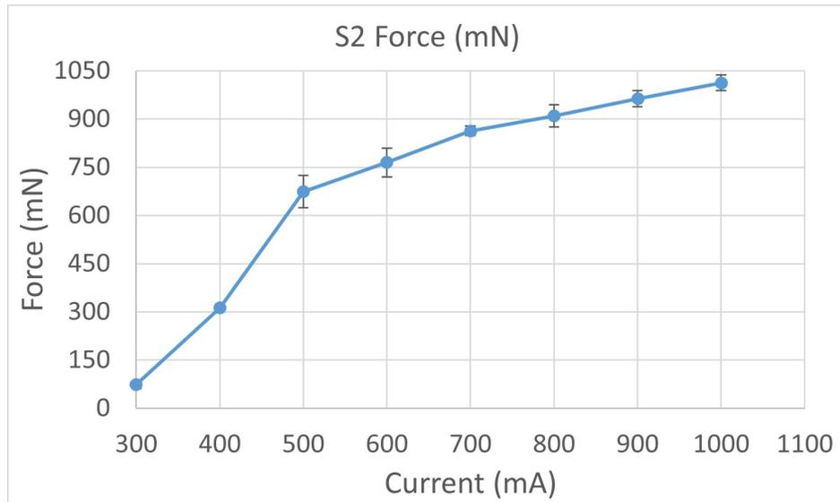
Figure 5.14: Force analysis of two-way SMA spring actuator - variation of forces for Spring 2 (S2)
