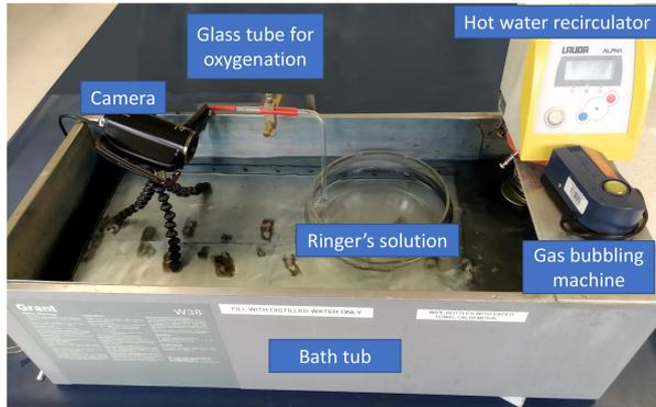
Fig. 9. In-vitro experimental setup to maintain peristaltic movements of ex-vivo intestine.
