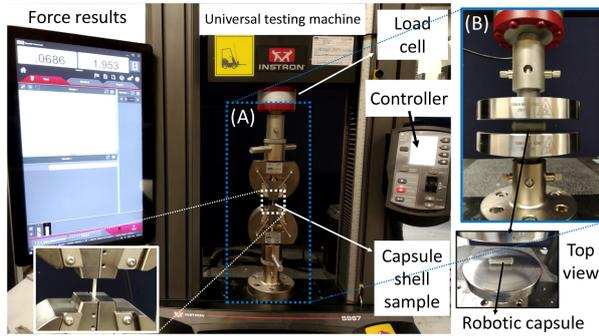
Fig. 2. Universal Testing Machine. (a) Tensile strength measurement of bio-compatible materials for capsule fabrication. (b) Actuator force output measurement of robotic capsule under various sealing mechanisms.
