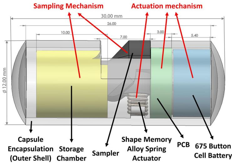
FIGURE 1 CAD-based concept design of capsule robot. PCB, printed circuit board
