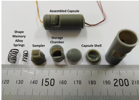
FIGURE 4 Capsule robot with 3D printed parts and shape memory alloy springs
