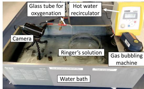
FIGURE 6. In-vitro experimental setup for postmortem tissue.
