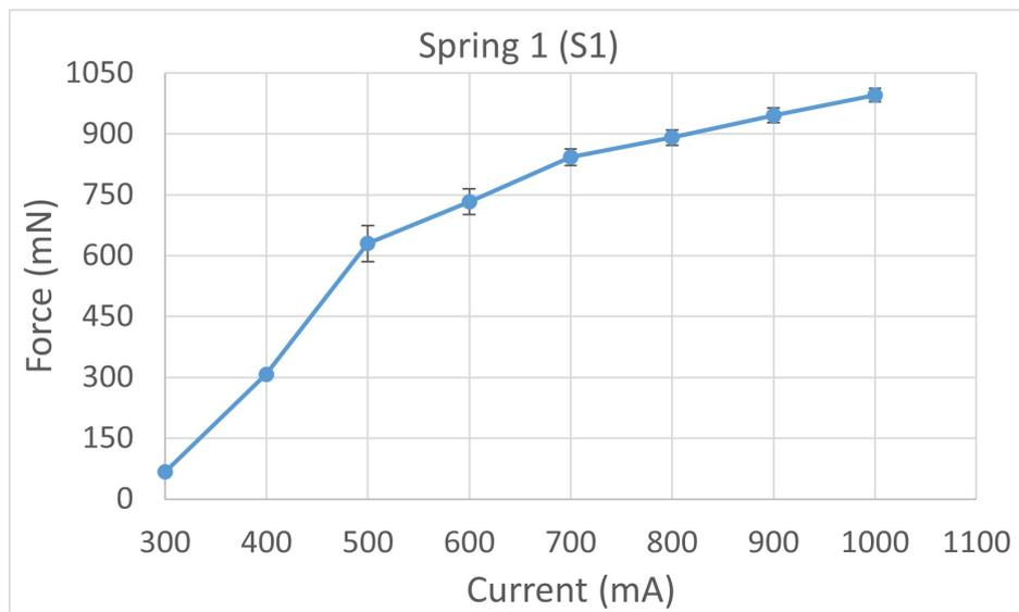
Figure 5.13: Force analysis of two-way SMA spring actuator - variation of forces for Spring 1 (S1)
