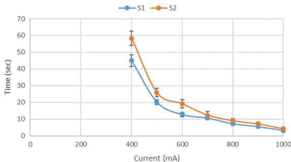
FIGURE 10 Actuation time for shape memory alloy springs
