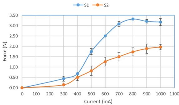
FIGURE 9 Force measurement of shape memory alloy springs
