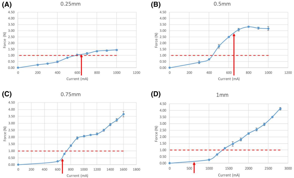
FIGURE 7 Force analysis for shape memory alloy springs with different wire diameters. Red arrow on x-axis indicates the maximum supply of current by a button cell battery (i.e., 650 mA). Red line on y-axis indicates the minimum required force to overcome intestinal forces (i.e., 1 N)
