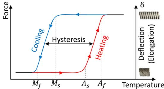
FIGURE 3. The relationship of force and deflection with different temperature states of SMA spring.
