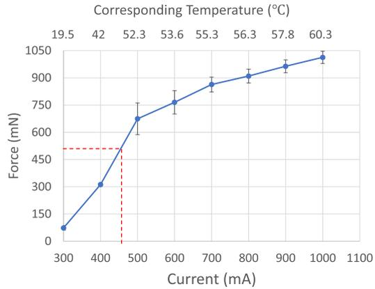
FIGURE 7. Force analysis of two-way SMA spring actuator.
