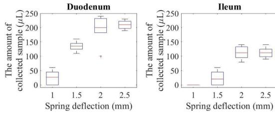
**FIGURE 11.** Variation in sample size collection by varying spring deflection on pig duodenal and ileal tissue.
