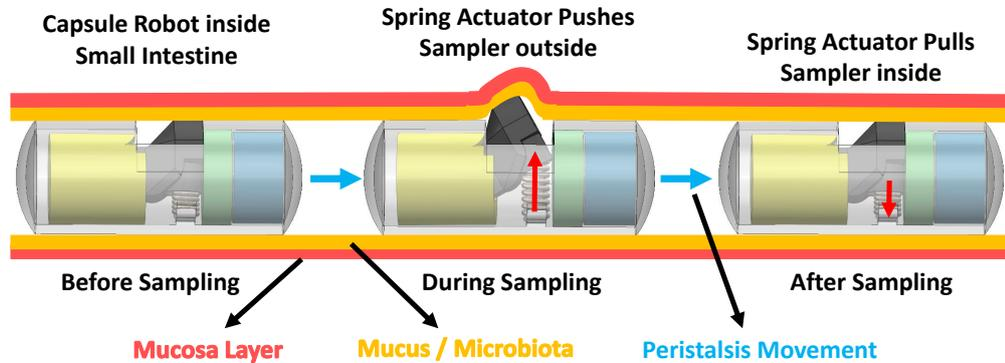
Figure 2.3: Dynamic sampling device that focus on collecting the microbiota from gut lining, image is reproduced from [75] © 2020 John Wiley & Sons Ltd.
