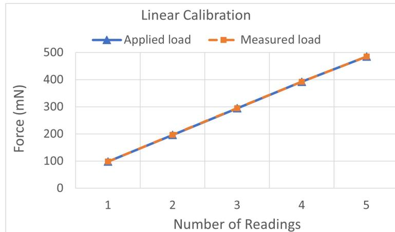
Figure 3.8: Linear calibration of the force sensor.
