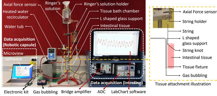
**Fig. 5:** In-vitro experimental setup for postmortem tissue with data acquisition systems for robotic capsule sensor and in-vitro axial force transducer. The intestinal tissue attachment inside the tissue bath chamber is elaborated separately on right side.
