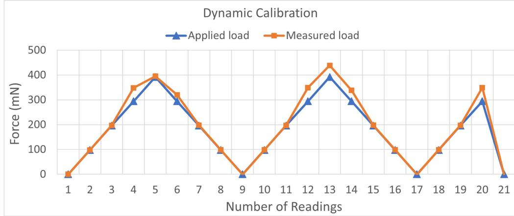
Figure 3.9: Dynamic calibration of the force sensor.
