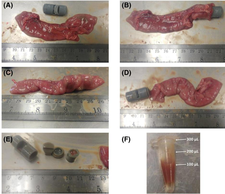
**FIGURE 12** Ex vivo experiments on the small intestine of a lamb. (A) The capsule robot and 100 mm section of small intestine, (B) the capsule entering the section of small intestine, (C) the capsule inside the small intestinal tissue, (D) the capsule exiting the section of small intestine, (E) the disassembled capsule parts and collected sample visible inside the storage chamber and (F) the sample is removed to an Eppendorf measuring tube
