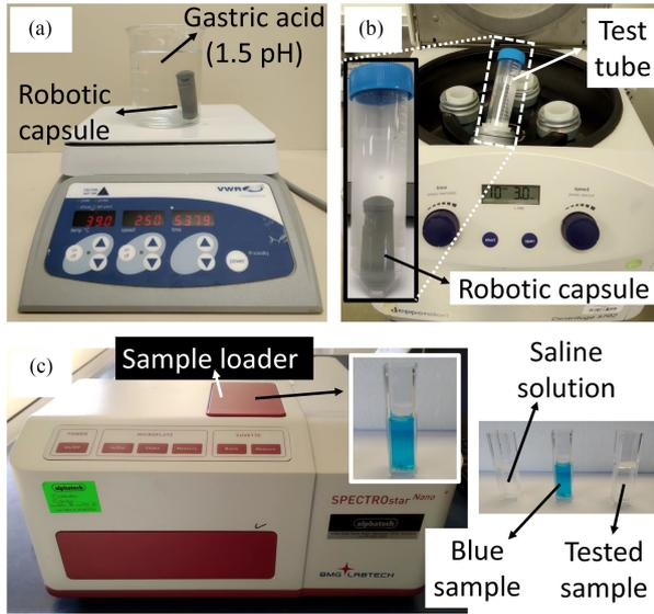
Fig. 4. (a) A magnetic stirrer machine used to replicate the stomach model and test the pre-sampling sealing mechanism. (b) A centrifuge machine to test the post-sampling sealing mechanism under agitation. (c) A spectrophotometer to analyse any potential leakage from the sealing mechanism.
