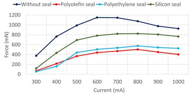
Fig. 7. Force analysis before and after sealing mechanism.
