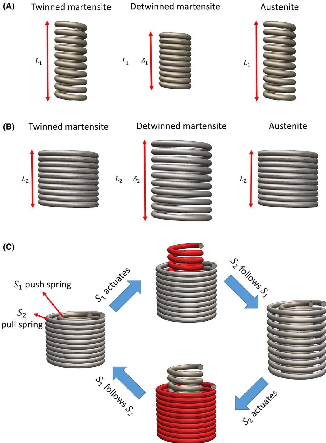
FIGURE 6 Shape memory alloy spring actuator. (A) Push spring S1. (B) Pull spring S2. (C) Antagonistic configuration with spring S1 and S2
