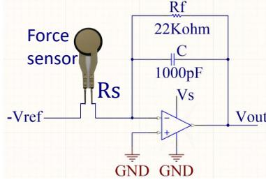
**Fig. 3:** Inverting Op-amp circuit for reading force measurements.
