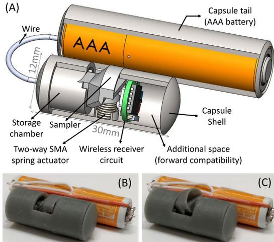
**FIGURE 1.** Robotic capsule prototype. (A) CAD model with AAA battery, an additional space (9 mm x  $\phi$  12 mm) is left to include high current drain button cell battery in future. (B) and (C) Fabricated capsule prototype with sampler closed and opened respectively.
