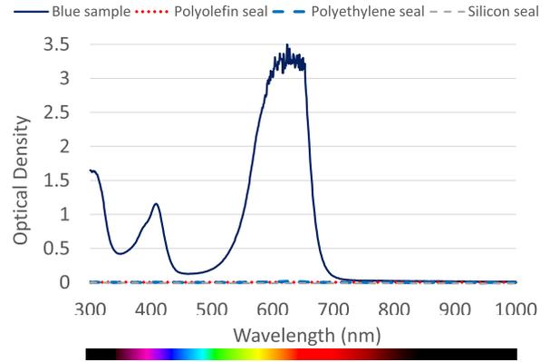
Fig. 5. Spectrophotometer results for the post-sampling sealing test under agitation conditions. The blue sample shows OD above 3 while all the three tested samples returned zero OD showing there was no leakage from the storage chamber.
