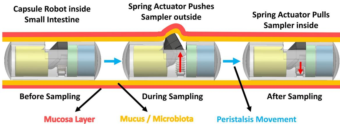
FIGURE 2 Sampling mechanism of capsule robot
