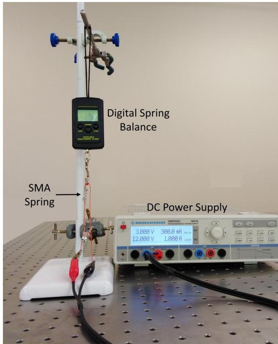
FIGURE 8 Experimental setup for force measurement
