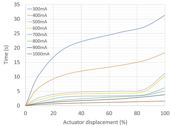
FIGURE 8. SMA spring actuator response time on varying currents.
