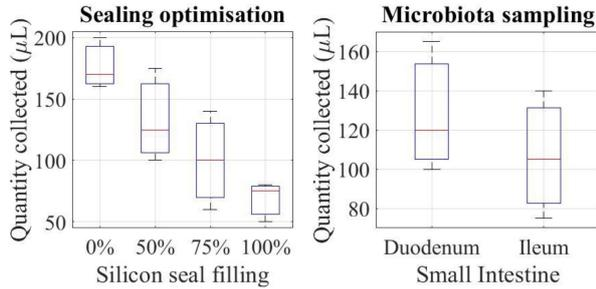
Fig. 10. (Left) Optimisation of filling percentage for the silicon seal of robotic capsule under intestinal trials. (Right) Sample collection from duodenal and ileal tissue after optimisation.
