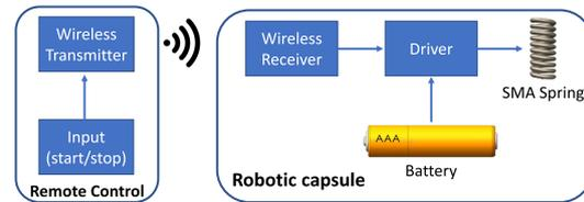
FIGURE 5. Electrical system design of the robotic capsule.
