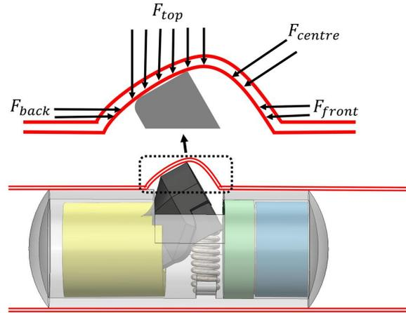
FIGURE 5 Intestinal forces on the sampler
