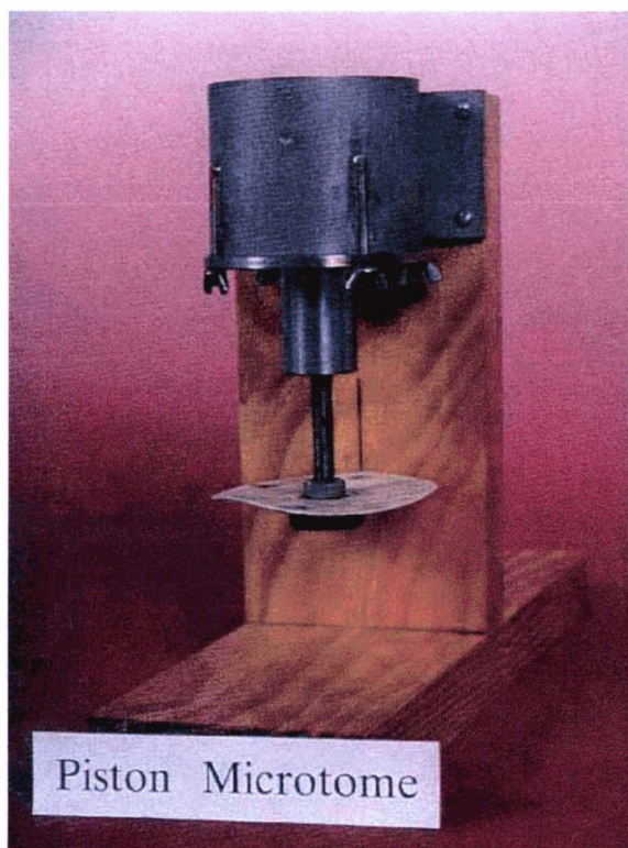
Plate 5.3 The piston microtome used for slicing soils from the lower RSC.
