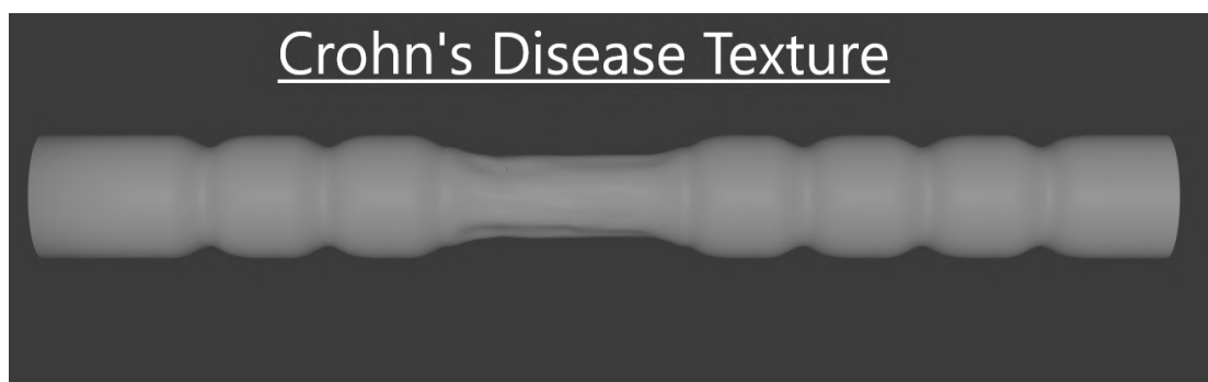
Figure 3.12: The textured surface that was added to the technical model using sculpting tools in a CAD package.
