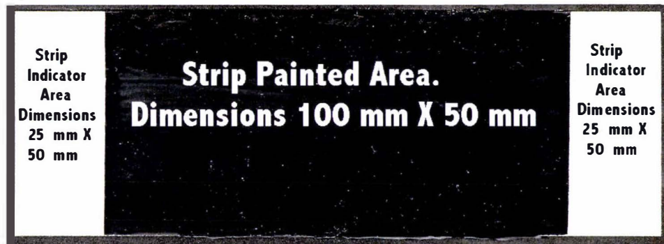
Figure 2.2: The structure of an oestrus detector strip.
