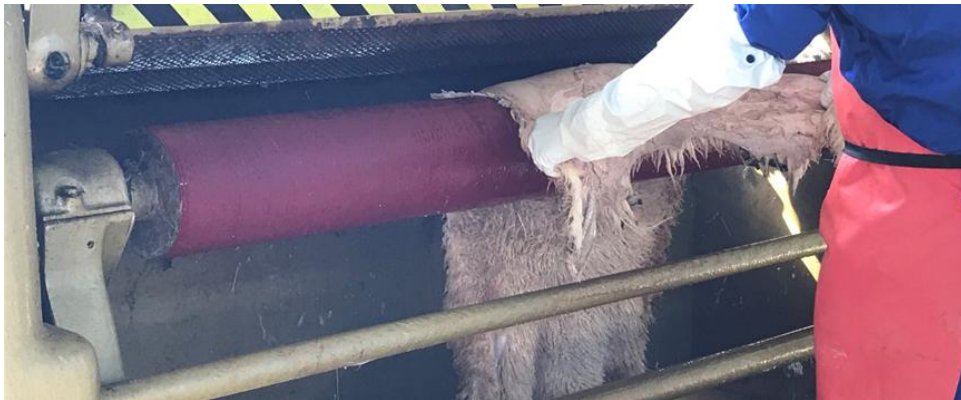
Figure 4.3 Removal of the fleshing layer by the hydraulic fleshing machine
