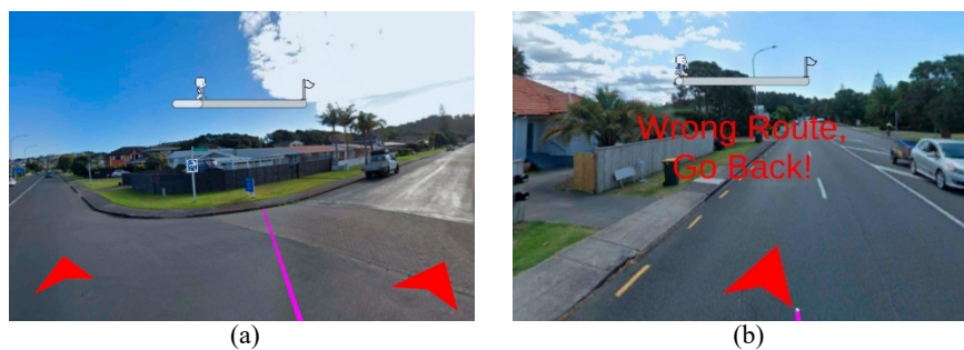
Figure 5. (a) Directional arrows as the navigation options available for users; a progress bar displays the evacuation progress. (b) Immediate feedback is given to users to turn around and get back to the best evacuation route.
