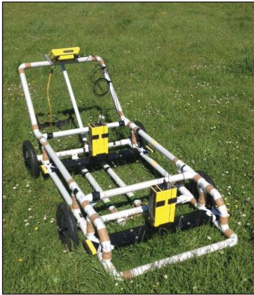
Figure 3.9: GPR setup showing the 100 MHz antennas with battery packs and display screen assembled on a PVC cart
