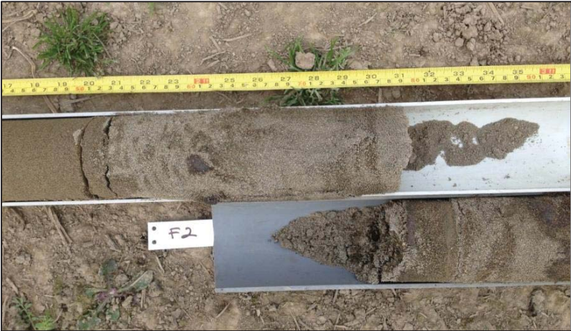
Figure 3.13: Measuring and labelling core lengths. Cores were collected in half – round PVC pipe for ease of movement off the Giddings rig.
