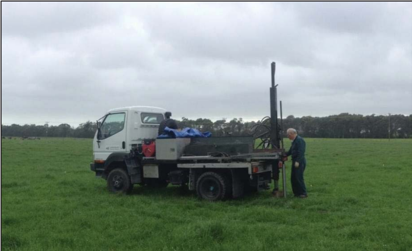
Figure 3.12: Giddings rig corer with soil corer attached.
