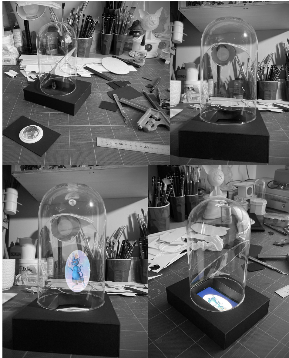
(Fig. 31) Prototype #2, Pepper's Ghost - digital projection concept.
