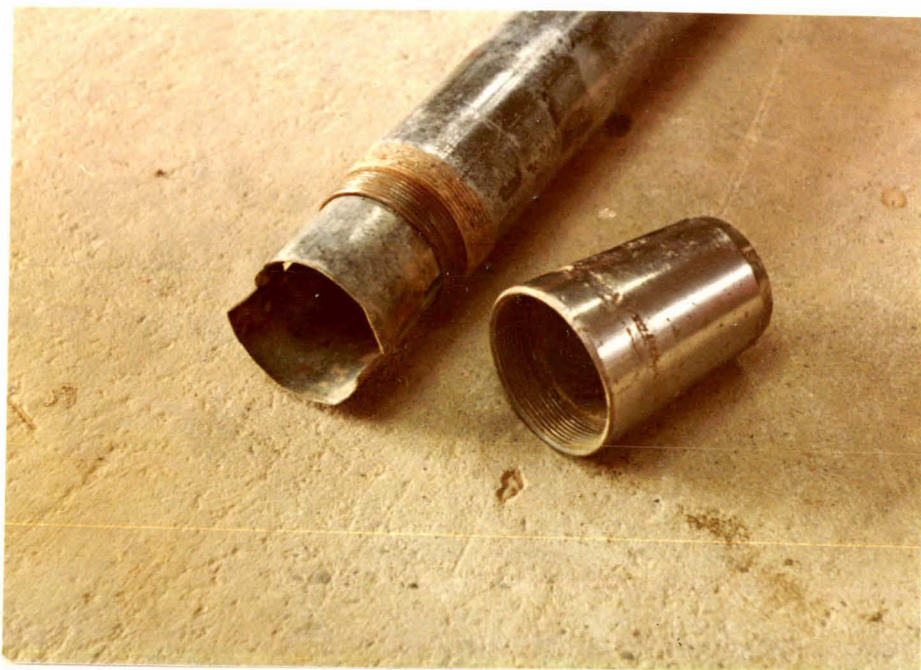
Plate 2. Close-up of cutting head and inner liners at base of corer.
