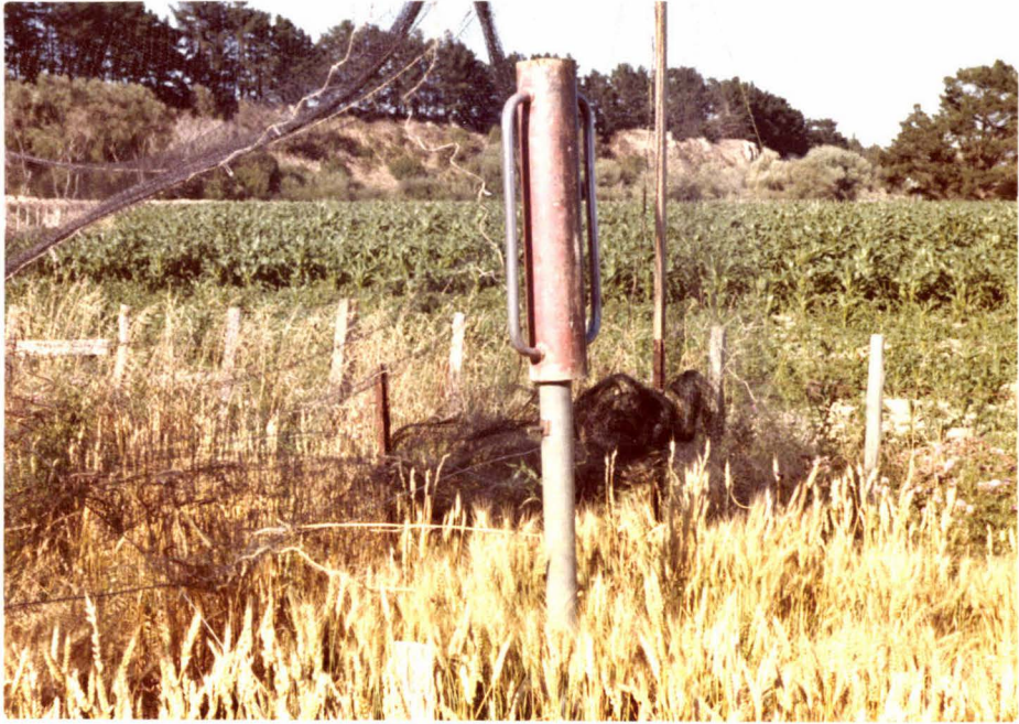
Plate 3. The corer in the plot with hand-rammer.
