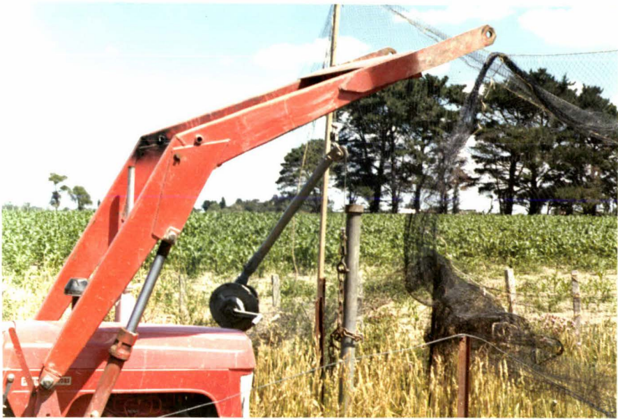
Plate 5. Removal of corer from soil using a winch.
