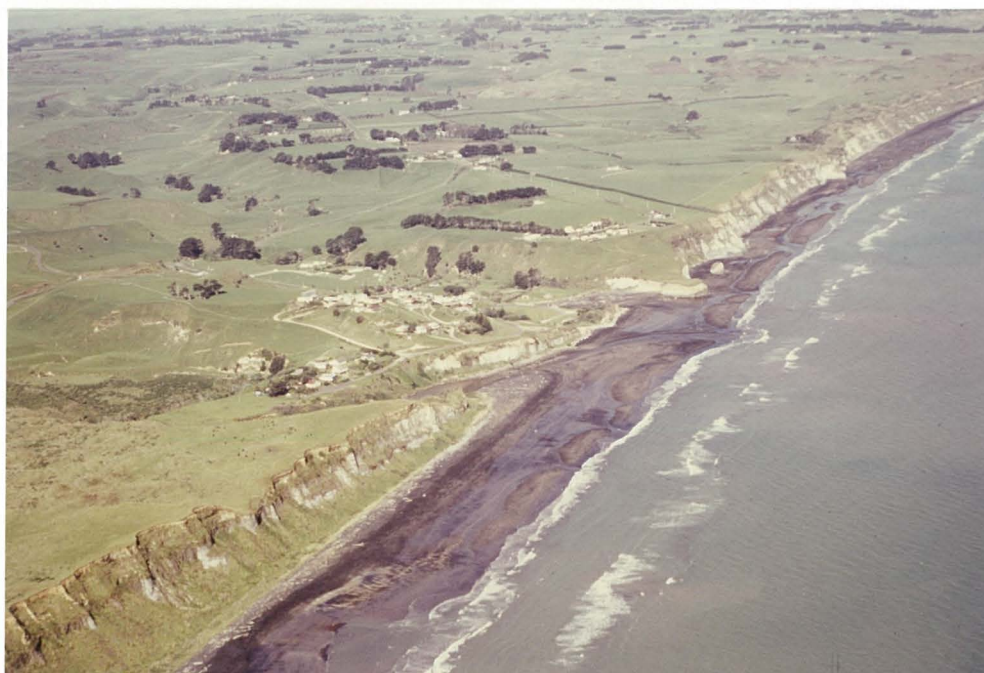
(Plate.3). Looking south along Kai-Iwi Beach with Mowhanau in the centre, showing Kai-Iwi (nearer) and Mowhanau Streams with eroding Castlecliffian cliffs south of Mowhanau. The cliffs of Nukumaruan age immediately to the north of Kai-Iwi Stream are partly protected by a small foredune built up at the toe of the cliff. The photograph was taken at low tide.
