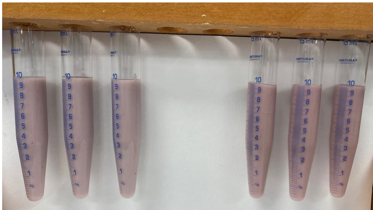
Figure 3 Visual stability test on day 1 showing 3 w/w% (left) and 5 w/w% (right) oleogel emulsions.
