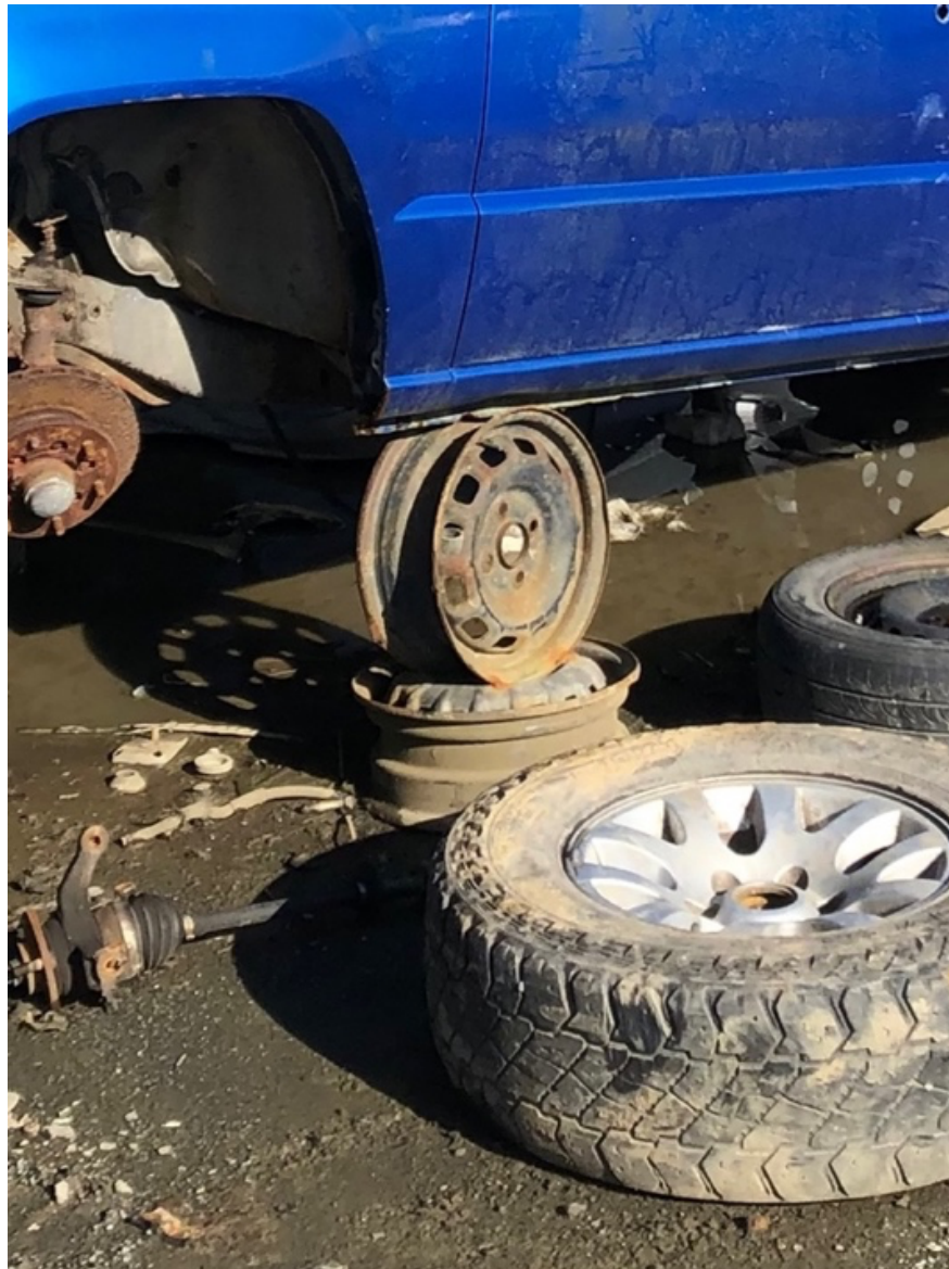
Figure 32: Two car rims welded together to form a car stand at Pick-A-Part car wreckers, 2023.
