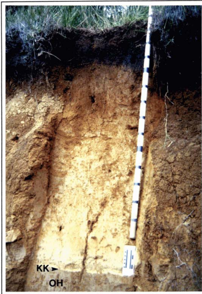
Plate 4.8 Kawa kawa Tephra at WF5. Note the thin fine-grained ash base to the Tephra (arrowed). Immediately underlying is yellowish-grey Ohakean loess (OH). Fine-grained rhyolite ash, which dominates the pale coloured coverbeds overlying the base of the tephra, grades upwards into Ohakean loess at the level of the base of the Jacob Staff. Ohakean loess grades upwards into the distinctive yellow-brown Holocene allophanic soil at c. 0.6 m from the base of the Staff. Both photograph 4.7 (previous page) and 4.8 courtesy of A. S. Palmer, Massey University.
