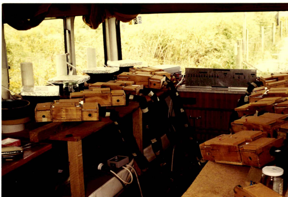
Figure 6.3. Arrangement of 10 observation hives, traps, tunnels and electronics, inside caravan (1987).
