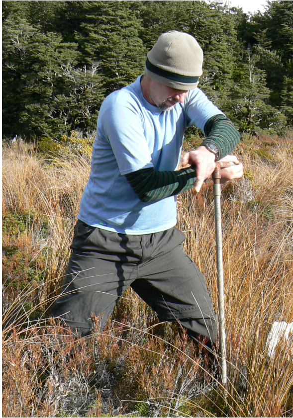
Figure 6.2: Piezometers being installed in the Tussockland community on 5 June 2007 at Silica Rapids Mire, Tongariro National Park.
