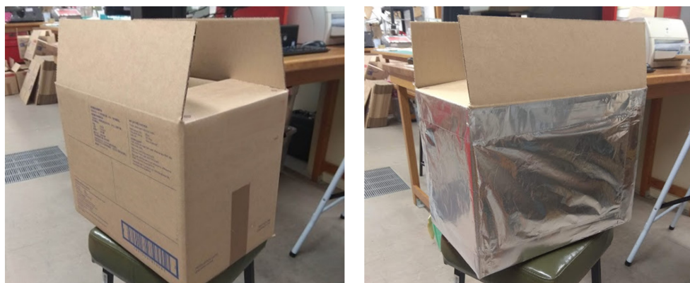
FIGURE 2 Assembled box with two normal panels (A) and aluminium foil covering two adjacent panels (B), the top flaps of the box were sealed with tape after the aluminium foil was applied
