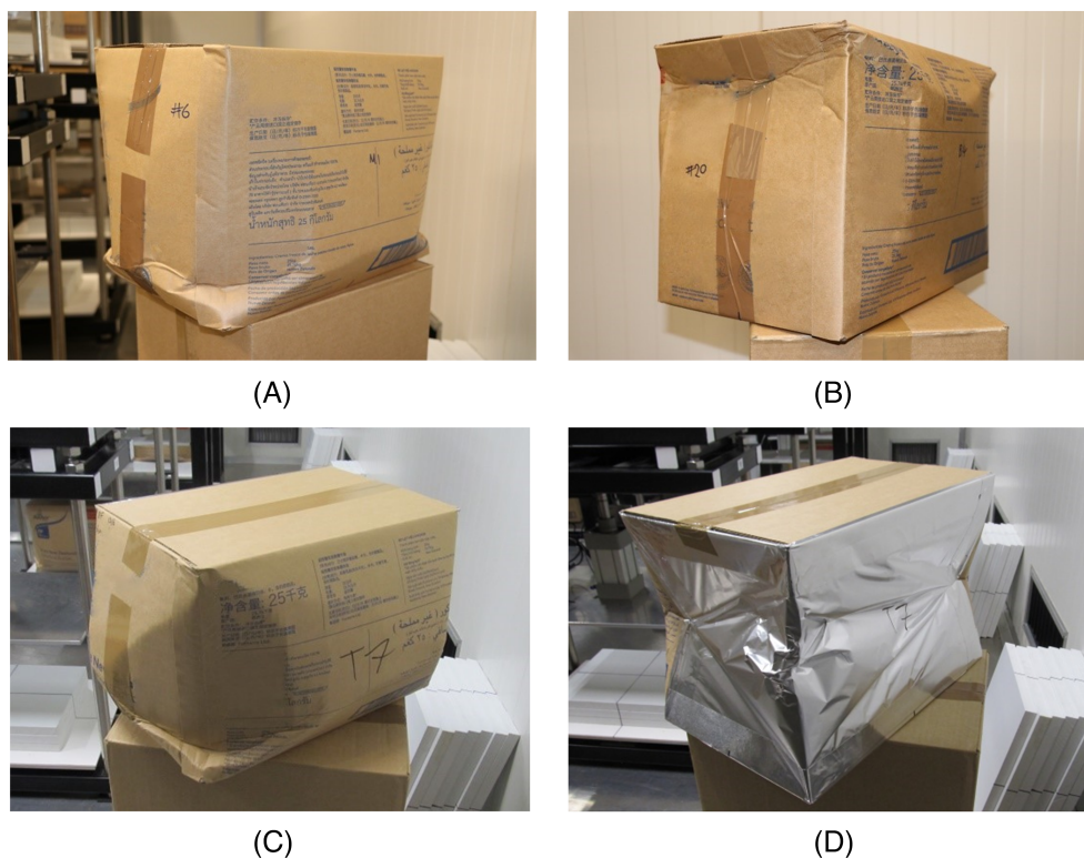
FIGURE 4 Manifestations of box failure as a result of creep deformation observed in this study: (A) and (B) show all panels of a control box in which it can be seen that creases and hinges form at the corners of the box which leads to buckling and global failure; (C) and (D) show the panels of a foil box, where similar creases and hinge formation is observed while the foil coated panels moved inward, this was observed for all foil boxes which failed
