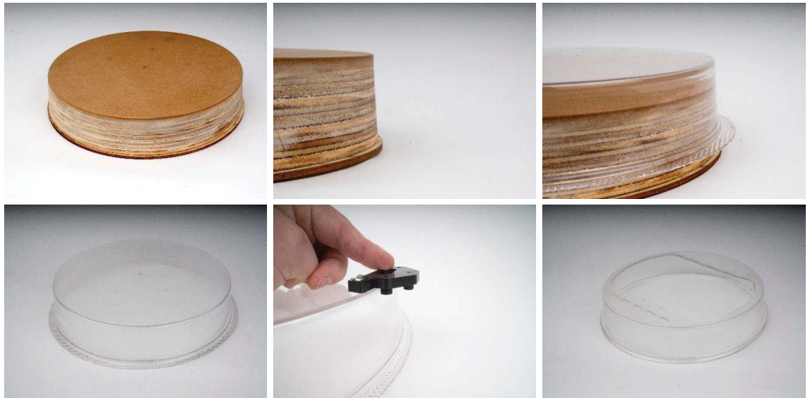
Image 60: Exploration of vacuum forming.
