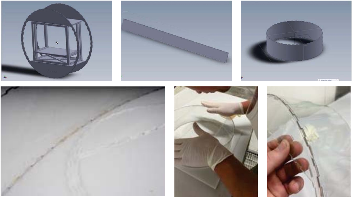
Image 50: Gluing PETG roll axis running surface for bearings.
