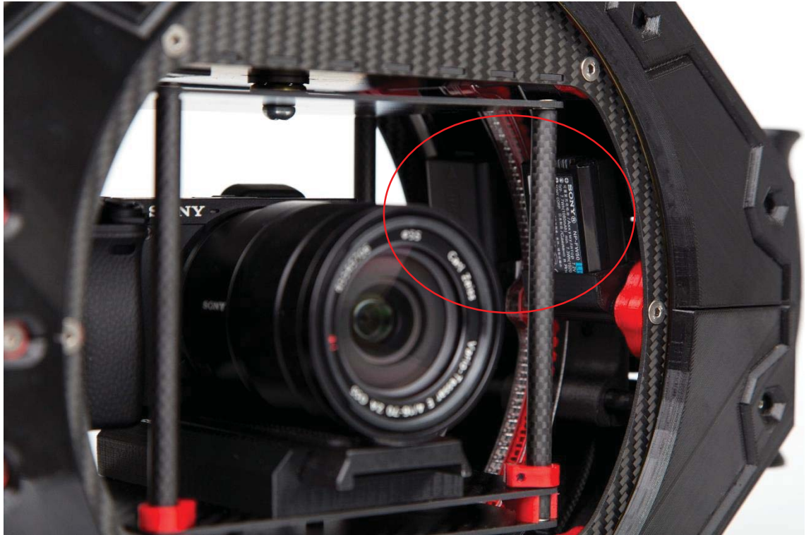
Image 90: Counterweights in roll axis.
