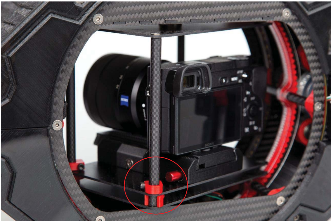
Image 93: Roll axis height - preset clips to maintain optical centre; camera safety release button.
