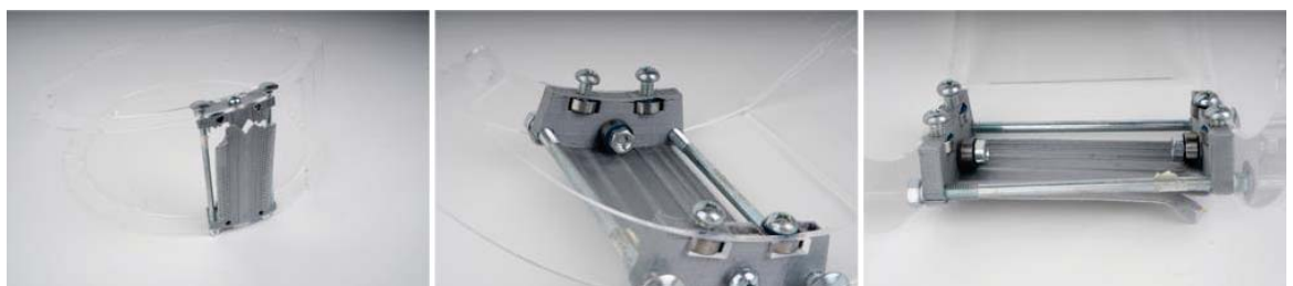
Image 40: Spacers and positioning of bearings.
