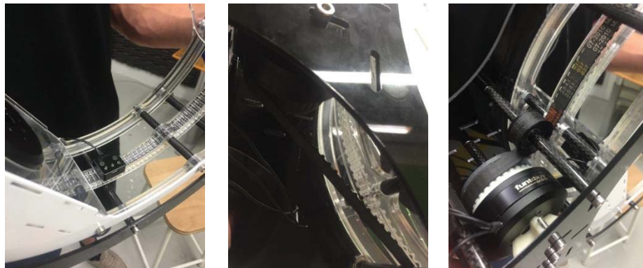
Image 68: Tensioning system for belt drive.
