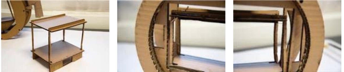
Image 23: Pan axis clearances.
