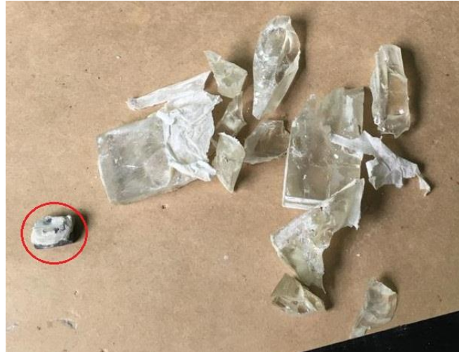
Figure 2.9 Sensor mount (circled in red) and 3D printed mold after producing the second cast prototype.
