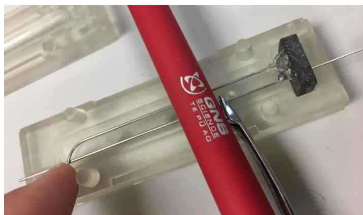
Figure 2.7 Placement of the sensor mount and internal tubing into the 3D-printed mold.
