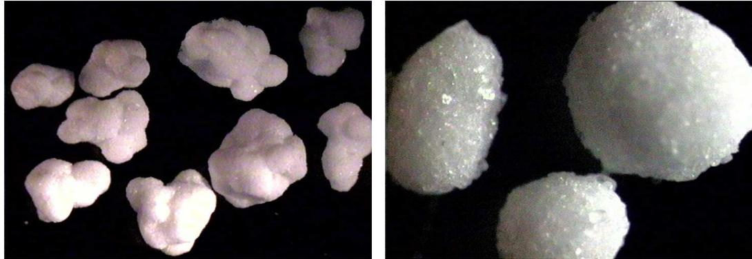
(a) Lactose granules formed using Polyethylene glycol (PEG) as the binder.
