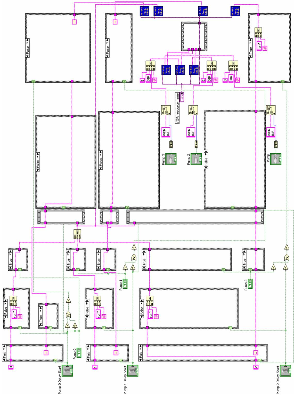
Appendix B. Core block diagram of VI to change pump settings.
