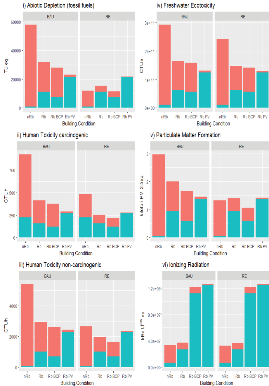
Figure 6.2 (b) The stock aggregated impact assessment results from 2017 - 2050 for buildings in four different conditions (nRb, Rb, Rb BCP, Rb PV) and two scenarios (BAU & RE) are shown for :i) Abiotic depletion (fossil fuels) ii) Human toxicity (carcinogenic) iii) Human toxicity (non-carcinogenic) iv) Ecotoxicity (freshwater) v) Particulate matter formation and vi) Ionizing radiation. The blue and red shaded areas represent the impacts embodied in construction and operational energy consumption respectively.
