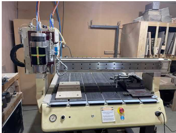
Figure 3.13 – CNC machine used to create known coordinate points
