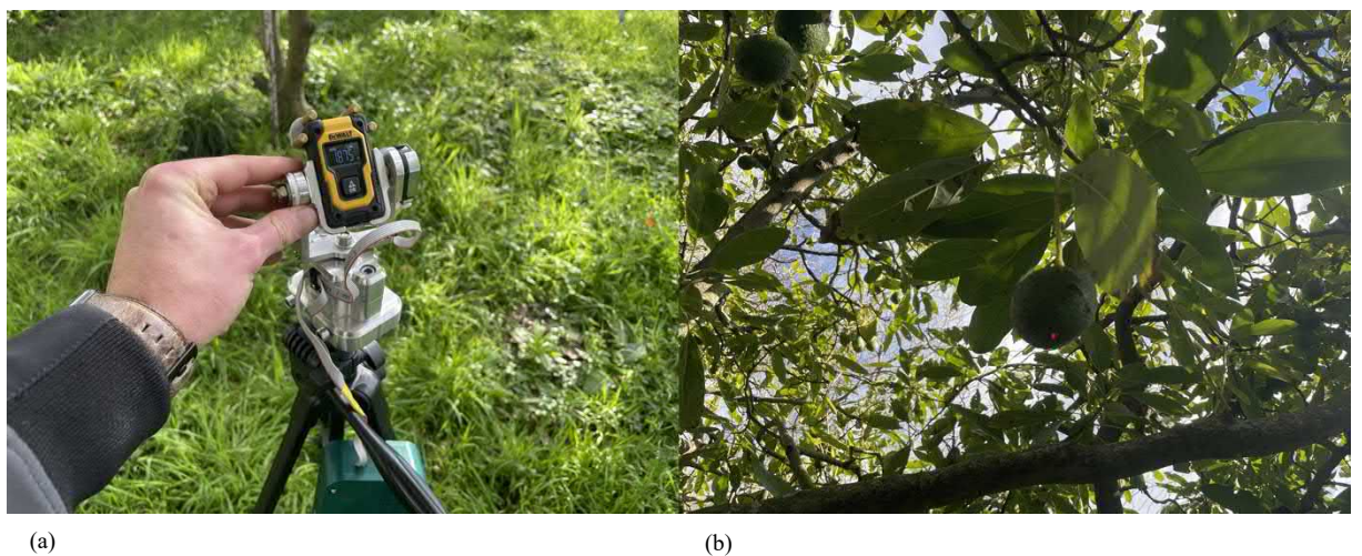
Figure 3.21 – Aiming the CMD by hand at a target avocado (a). Laser dot visible on the base of an avocado (b)
