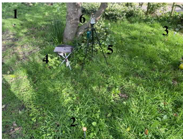
Figure 3.20 – Trial measurement setup with datum points (1, 2, 3), data collection PC (4), tripod (5), and CMD (6).
