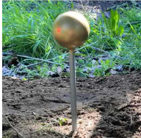
Figure 3.32 – Aiming the laser dot at the centre of the datum point for an accurate measurement
