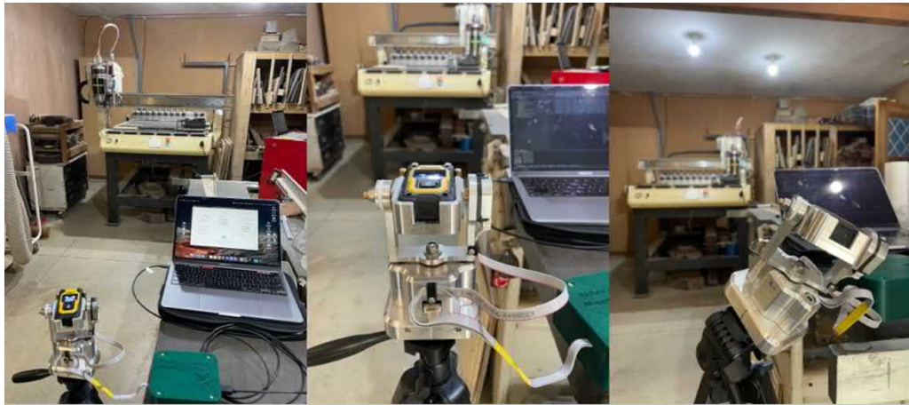
Figure 3.14 – Measuring positions of CMD from three different arbitrary orientations
