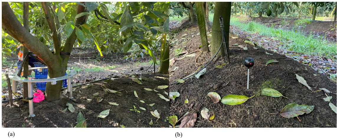
Figure 3.29 – Datum points placed around frame setup (a). One datum placed on the raised bed for greater tripod visibility (b)
