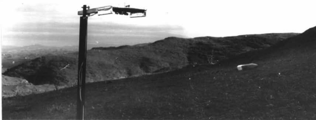
FIGURE II.7 Sensor Unit for 120 cm. Air Temperature Measurements.
