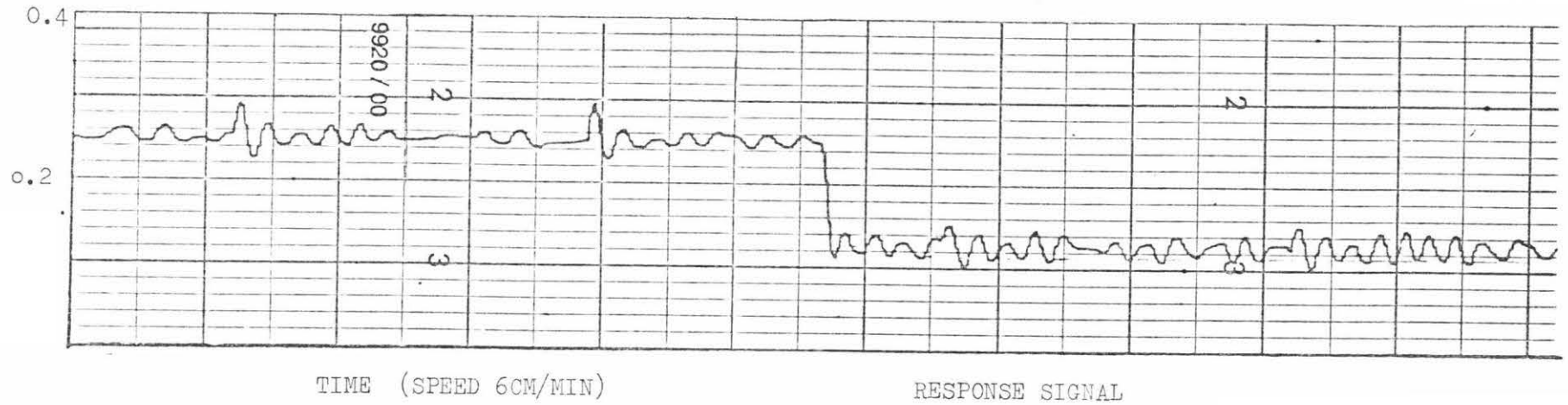
Fig. 4.4 Set-point changes under first set of sensors with controller in action when web system is in progress.
