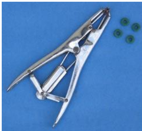
Figure 2. An example of an elastrator, the device used in this study to apply a tight rubber ring to the neck of the scrotum (castration) or the base of the tail (tail docking). Photo taken from http://www.luresext.edu/photos/elastrator.jpg .
