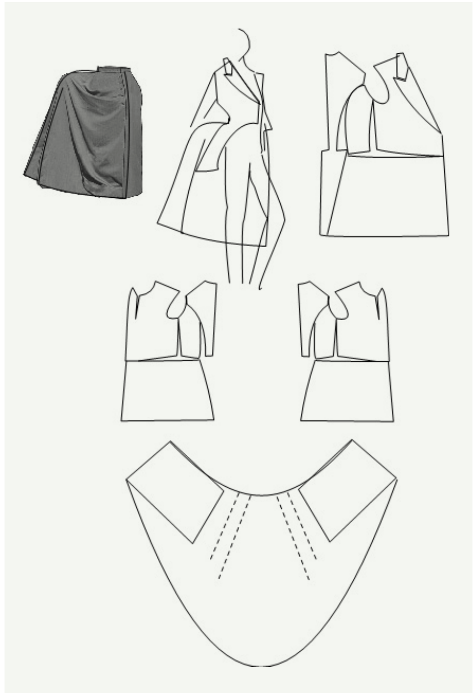
RIGHT Figure 155. Pattern development and working drawings for 'Riding-on suit'. Author's own (2010)
