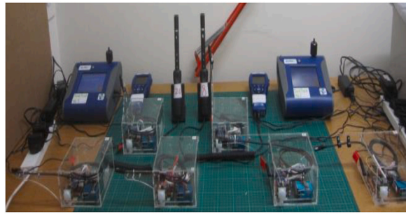
Fig. 4. Experimental setup for the controlled location of the pre-fieldwork validation study of SKOMOBO platforms with reference platforms. Six SKOMOBO sensors were enclosed in a clear acrylic frame and reference platforms (two TSI Q-Trak 7575, TSI Incorporated, Shoreview, Minnesota, USA) co-located in controlled office environments with a common area.
