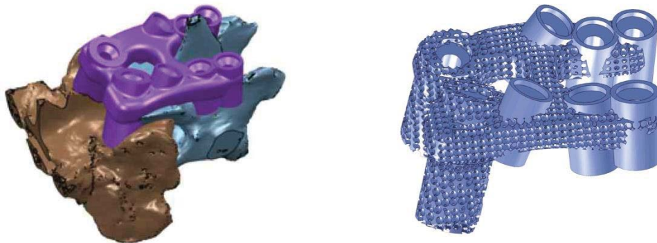
Figure 50. Computer generated 3-dimensional model of the LS junction of a dog with DLSS. The custom designed implant for dorsal stabilisation is in purple, the sacrum is in brown and L7 is in grey. On the right the implant has been rendered into a porous titanium scaffold with screw turrets that guide screw application in pedicles of L7 and the sacrum.
