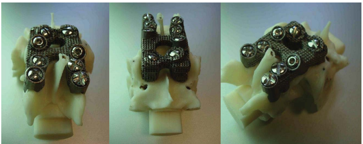
Figure 48. Computer designed titanium implant mounted on acryl-nitrile butadiene styrene plastic renditions of L7 and the sacrum of a GSD.
