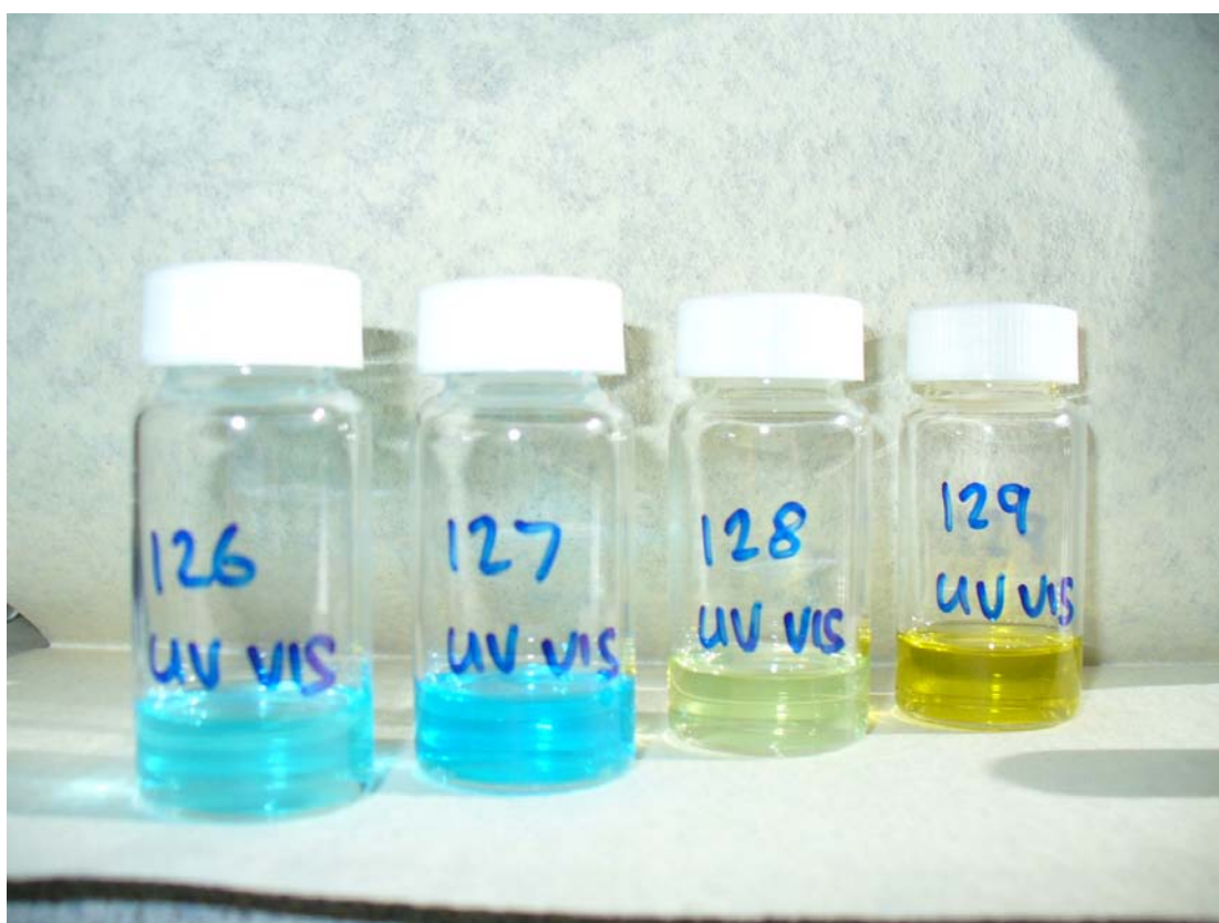
Figure 23 Samples in CH 2 Cl 2 of [NP(biph) 0.66 (2O-4-MePy) 0.33 ] n with, from left: CoCl 2 6:1, CoCl 2 2:1, CuCl 2 6:1, CuCl 2 2:1
