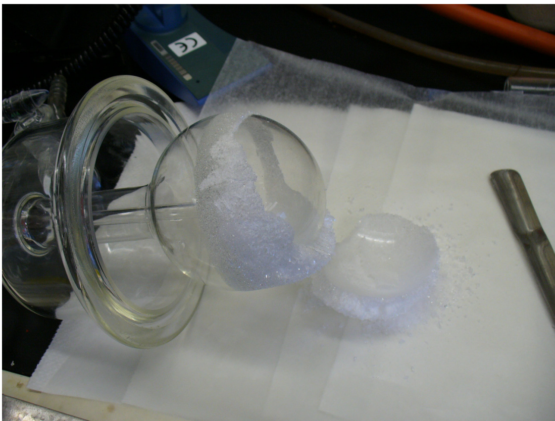
Figure 4 Removing the sublimed cyclochlorophosphazene
