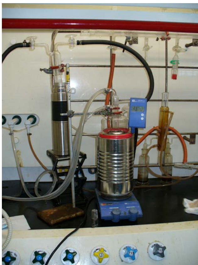
Figure 2 Sublimator setup in oil bath with cold trap
