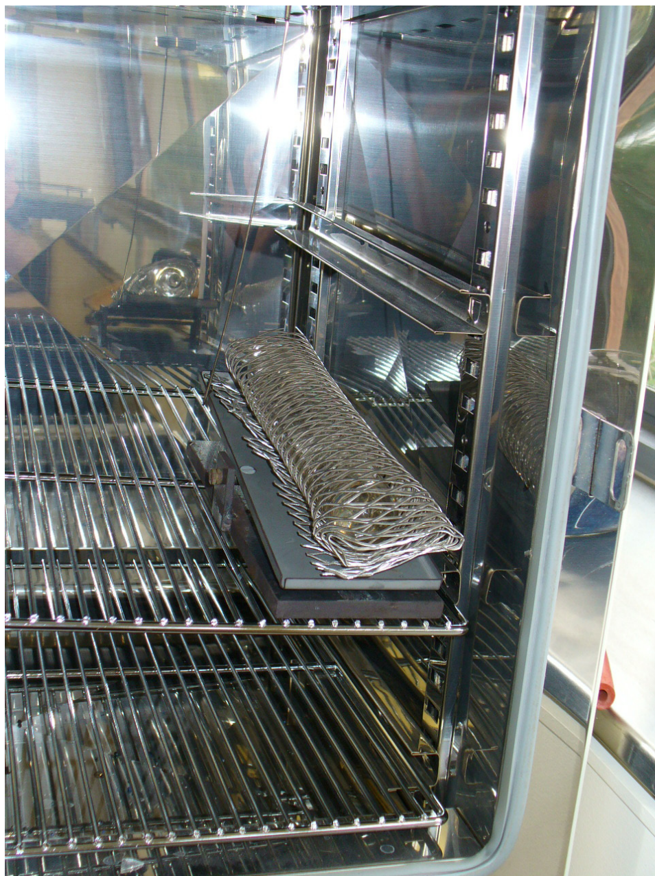
Figure 7 Reaction tube ready for thermal polymerisation
