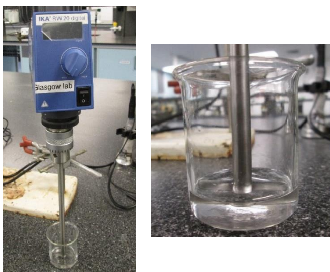
Figure 6.1: Set up of the stirrer for testing digestion in the stomach
