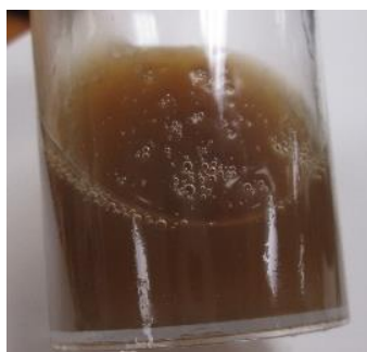
Figure 5.14: Image showing the mamaku + gelatin solution which was loaded into the syringe
