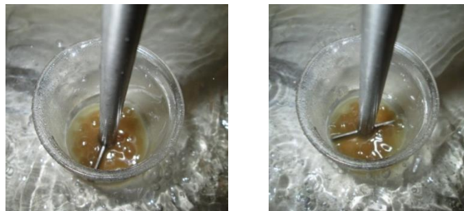
Figure P.1: Images taken before melting (left) and as the beads began to melt (right) as the sample was heated in the water bath
