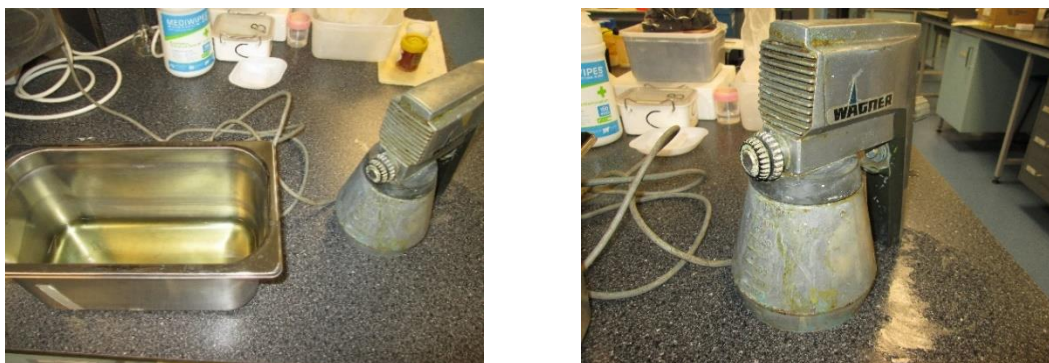
Figure M.1: Images showing the paint gun and set up of the cold oil bath
