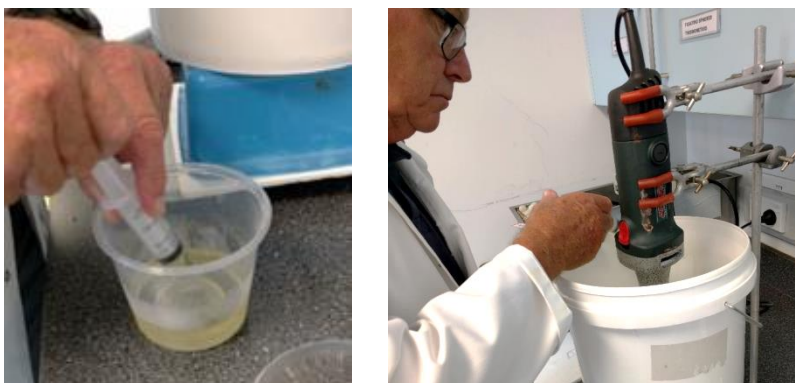
Figure N.1: Images showing loading the chilled oil into the syringe (left) and then distributing this cold oil around the sides of the bucket (right)
