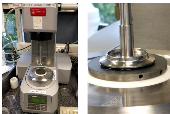
Figure 5.1: Pictures showing the set-up of the rheometer, including the cone and plate geometry with a sample loaded in
