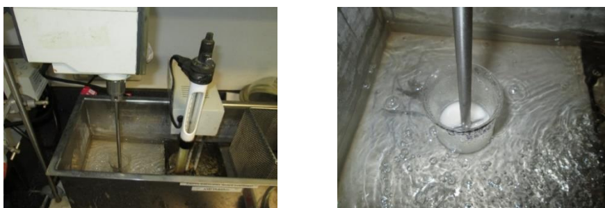
Figure 6.6: In-vitro digestion of the emulsion based encapsulated mamaku
