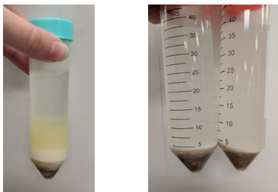
Figure 5.10: Image showing the layers created by centrifuging in the first cycle (left). Image showing the layers created by centrifuging in the last cycle (right).
