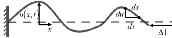
Figure 6: A bended filament with inextensible arc-length (contour length) l_C and one fixed end can be characterized by its transverse displacement from a straight conformation (dashed line). The transverse thermal fluctuations lead to a contraction of the end-to-end distance, which is denoted by \Delta l [39].
