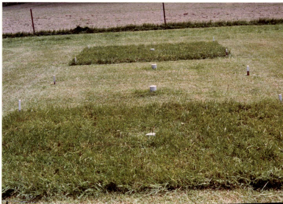
Plate 1. The cutting height pretreatments. Aluminium tins at the centre of each plot cover neutron probe access tubes.
