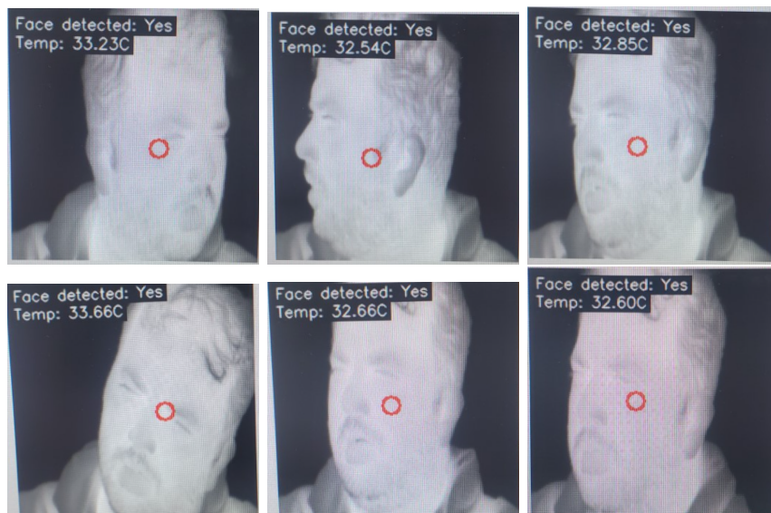
FIGURE 5.3: Sample frames with face detected, showing centroid and predicted temperature.
