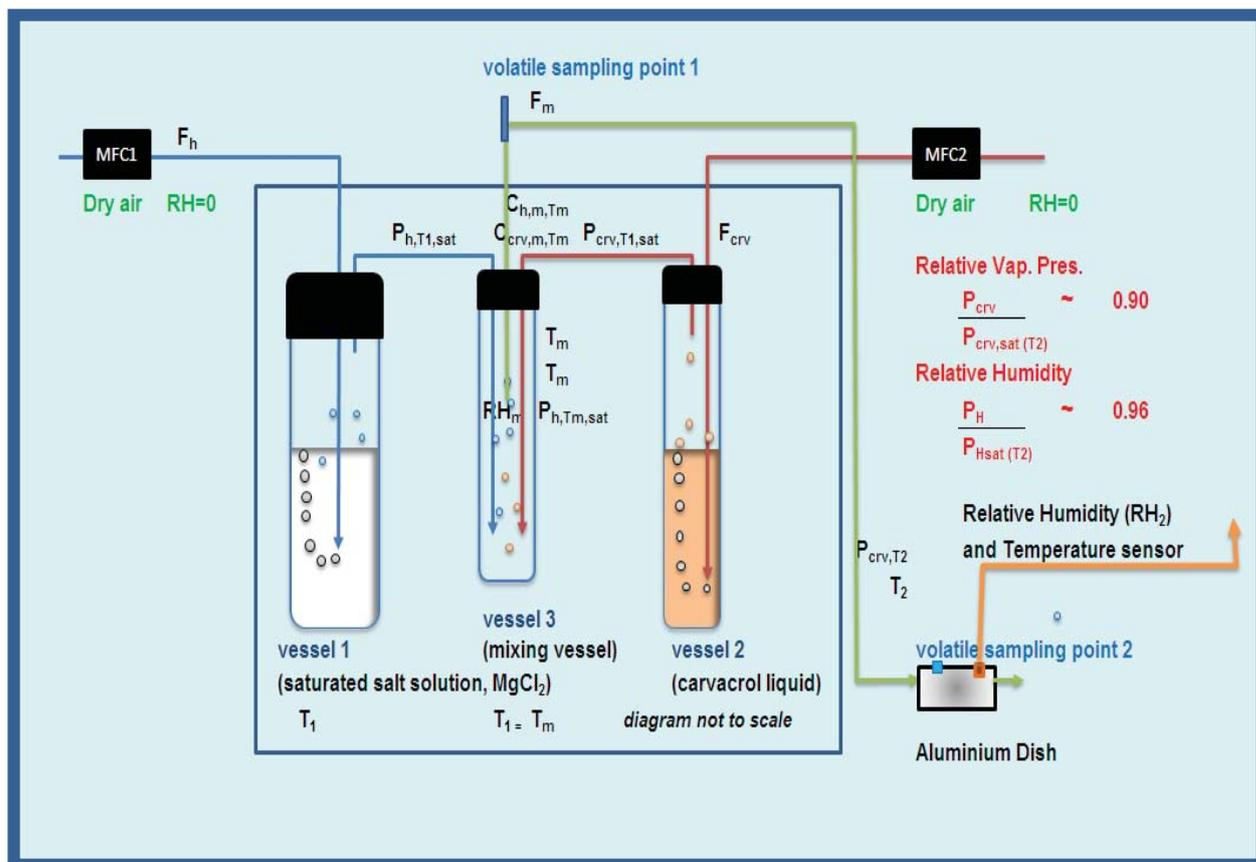
Figure 7-10: Schematic diagram of the volatile generating system.
