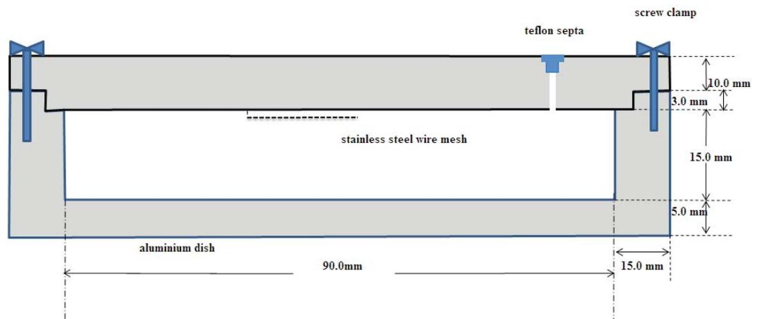
Figure 4-2: Schematic representation of the experimental aluminium dishes
