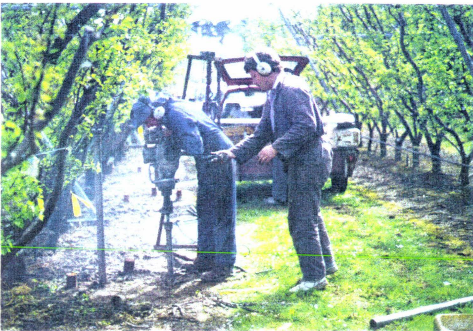
Plate 4.2 Root core sampling from close planted trees in early spring of 1992-1993 season. a). Selecting the best position for installing coring tube and equipment for sample 0.2 m from tree. b). Driving core tube into the soil using a modified engine-powered concrete breaker.
