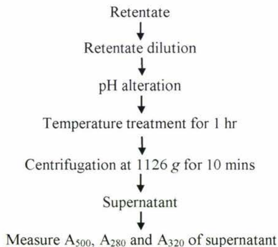
Figure 5.4 General experimental procedure for determination of the effect of selected variables on the flocculation and separation of MFG from retentate.
