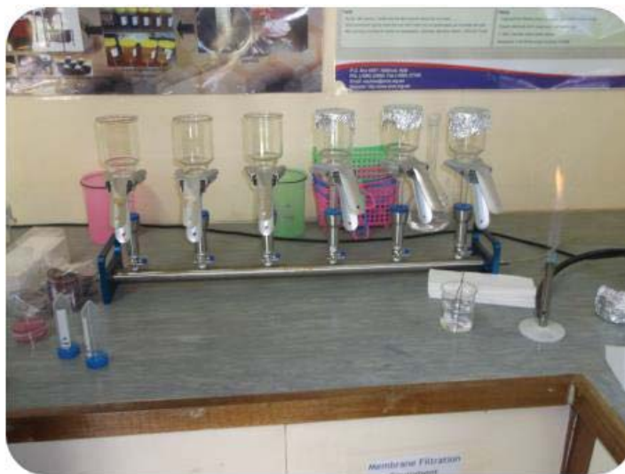
Figure 26. Preparation bench with standard equipment used for Total coliform and E.coli determination
