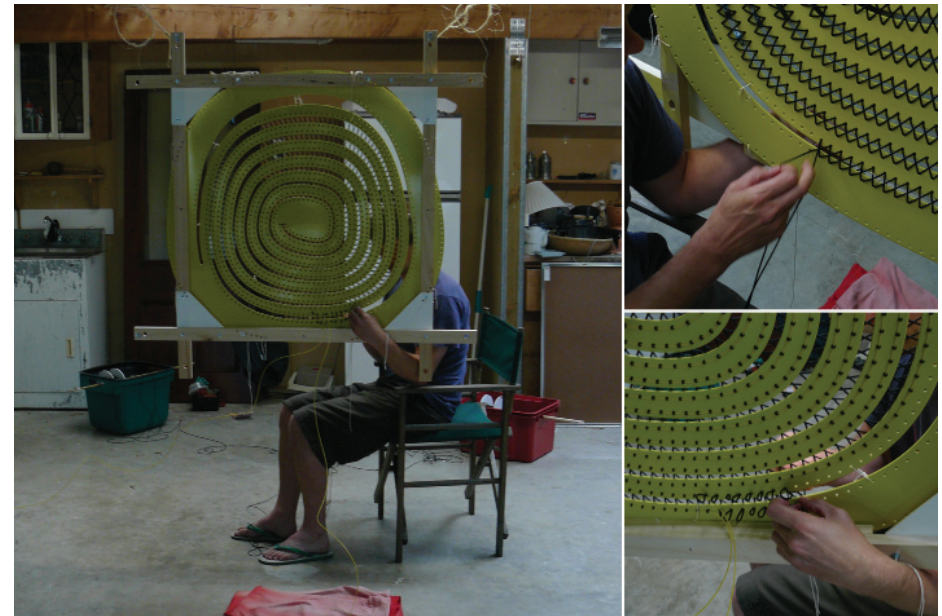
Figure 132 Hand stitching construction of 'Sprung'.
