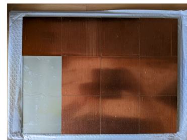
Fig. 4. Calibration board backside with partially applied copper plates.
