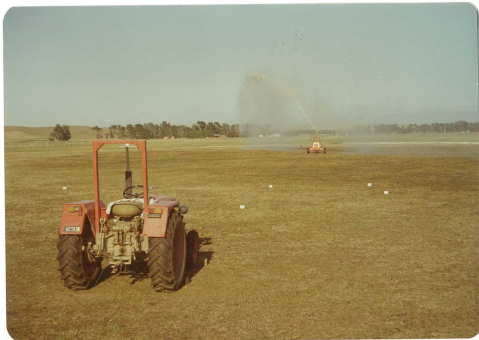
Fig.63 A photograph of the experimental site, showing the containers used for measuring the amount of water applied, and the "big gun" irrigator.
