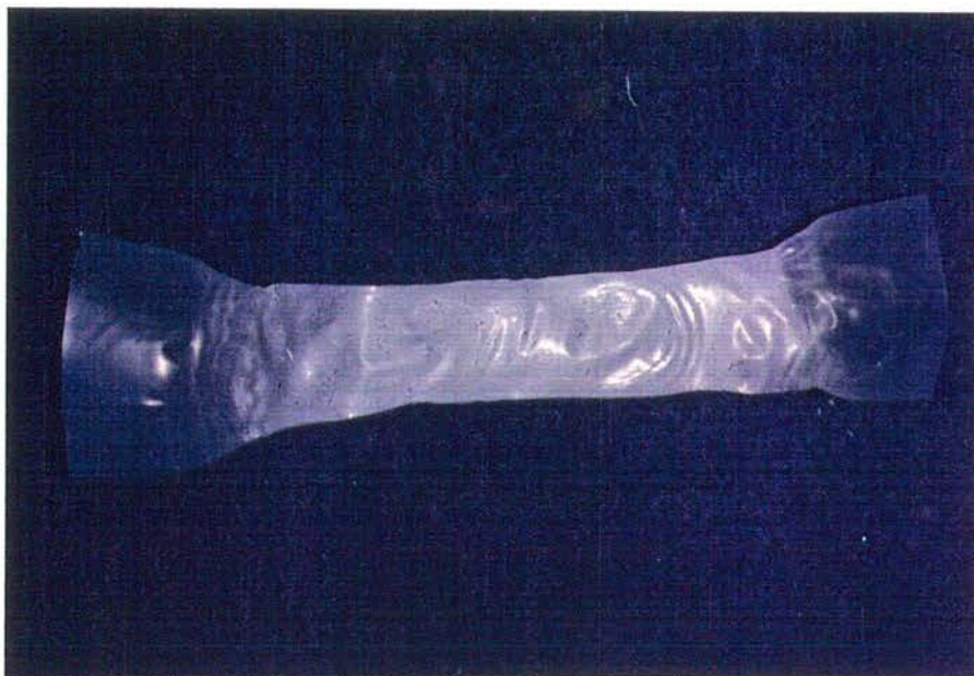
Plate 5.1 Infra-red polyethylene film sample after breach of the materials elastic limit
