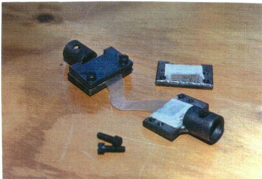
Plate 4.2 The gripping system employed for the tear resistance and tensile testing
