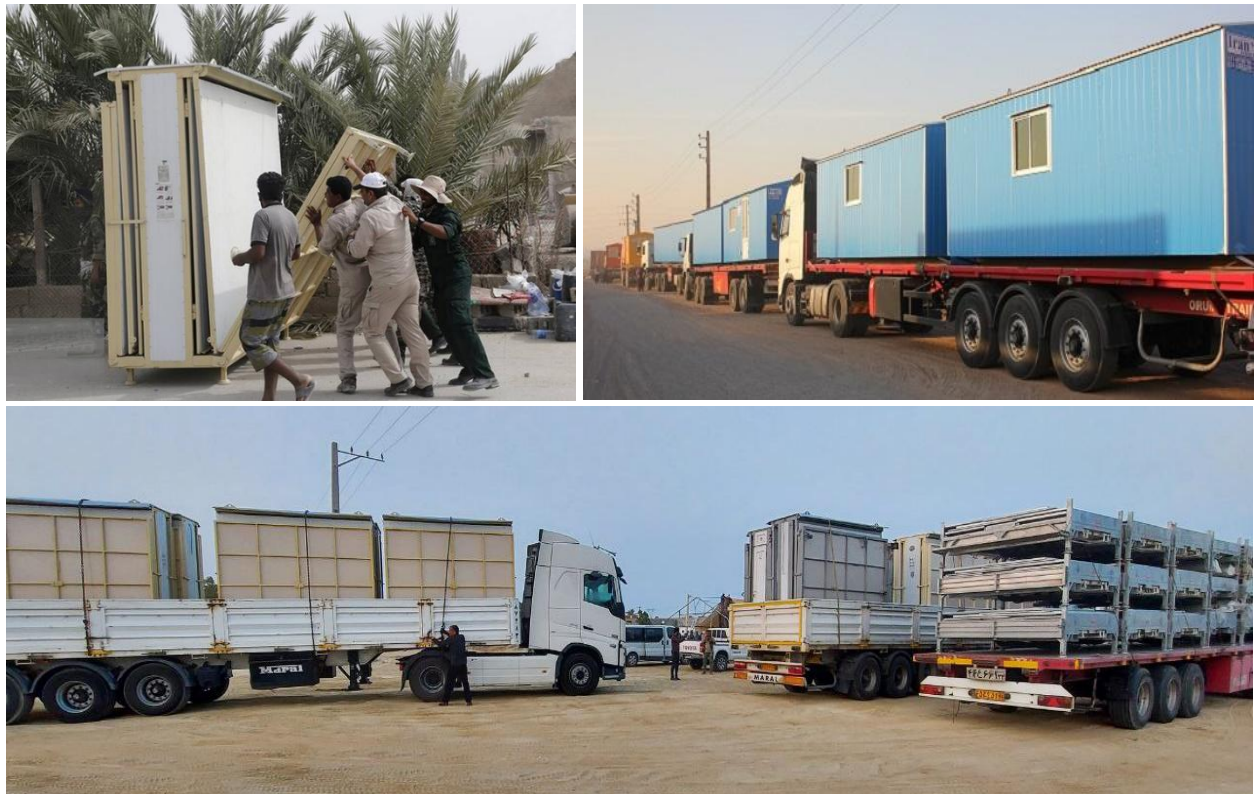
Figure 5.4. Top right: the bulky shape of the temporary housing units employed in previous disaster relief programs. Top left and bottom: the foldable temporary housing units used in Sayeh-Khosh village.
