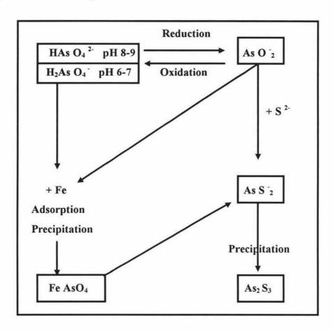
Figure 2.4 Chemical transformation of As in soils (Modified from Nriagu, 1994).
