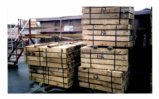
Plate 3.5 Freshly treated timber at the Carter Holt Harvey timber treatment plant, Marton (after steam drying).
