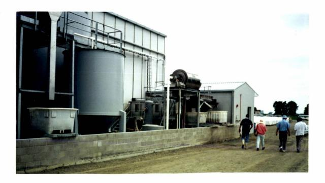
Plate 3.1 Chromium precipitation tank, used to recycle Cr into the tannery at J.D.Wallace tannery, Waitoa.
