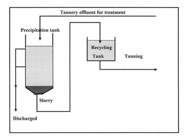
Figure 2.3 Chrome recycling drum system.
