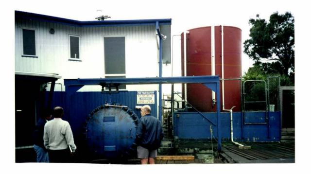
Plate 3.4 CCA treatment chamber with steam drying facility for drying the the freshly treated timber.
