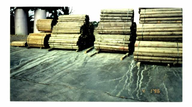
Plate 3.6 CCA drips from freshly treated timber in a timber treatment plant (without steam drying).
