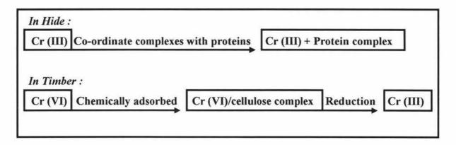
Figure 2.2 Simplified processes of Cr fixation onto hide and timber.
