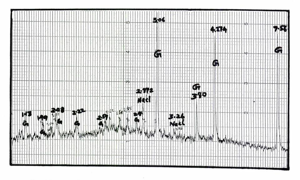
Figure 4.7 XRD pattern showing the peaks for gypsum -G - (CaSO 4. 2 H2O) and sodium chloride (NaCl).
