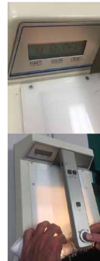
Figure 87. Opacity measurement of the lightest area printed self-adhesive film with UV transmission Densitometer X-rite 361T, personal photograph by Vivian Fei, 2021
