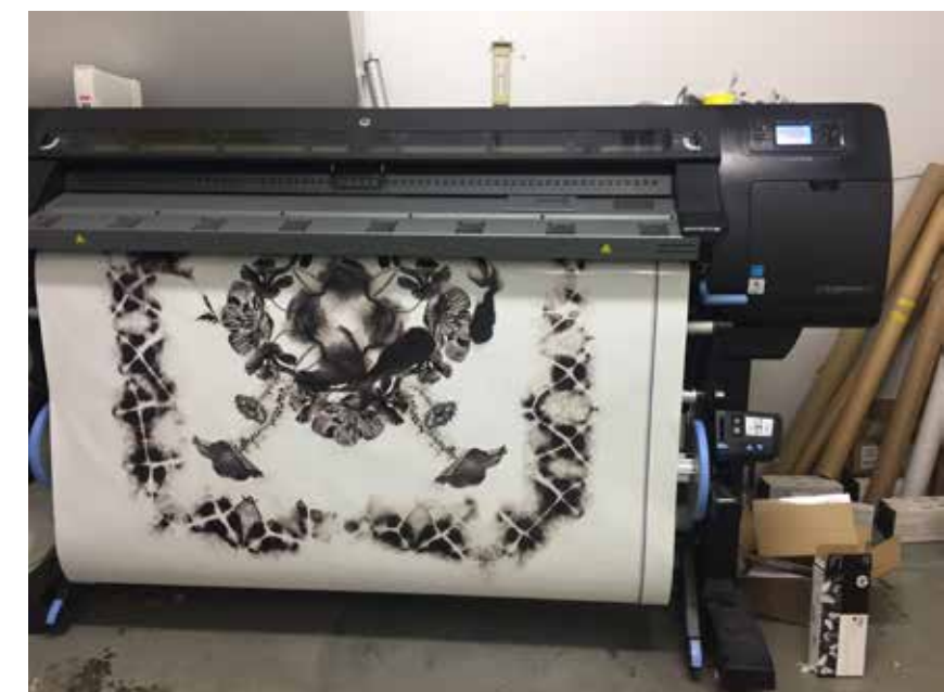
Figure 83. Digital negatives printing on self-adhesive film (Arlon 4500G clear, 1500mm width) in HP Designjet L26500 color inkjet printer with HP Latex Inks, personal photograph by Vivian Fei, 2020
