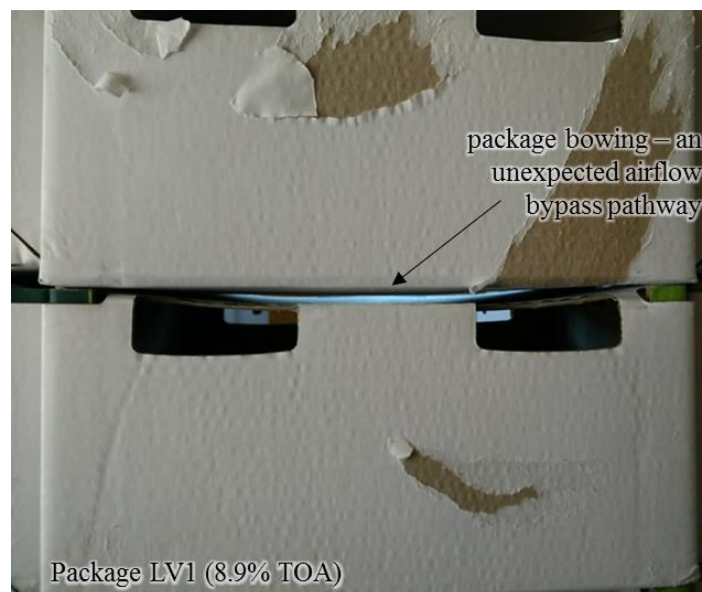
Figure 3.18: Package bowing as a result of weakened packaging, due to increased vent sizes. This created an unexpected airflow bypass pathway. Note that the tears on the packages are just superficial damage to the surface as a result of handling and thermocouple attachment. This does not represent structural damage.
