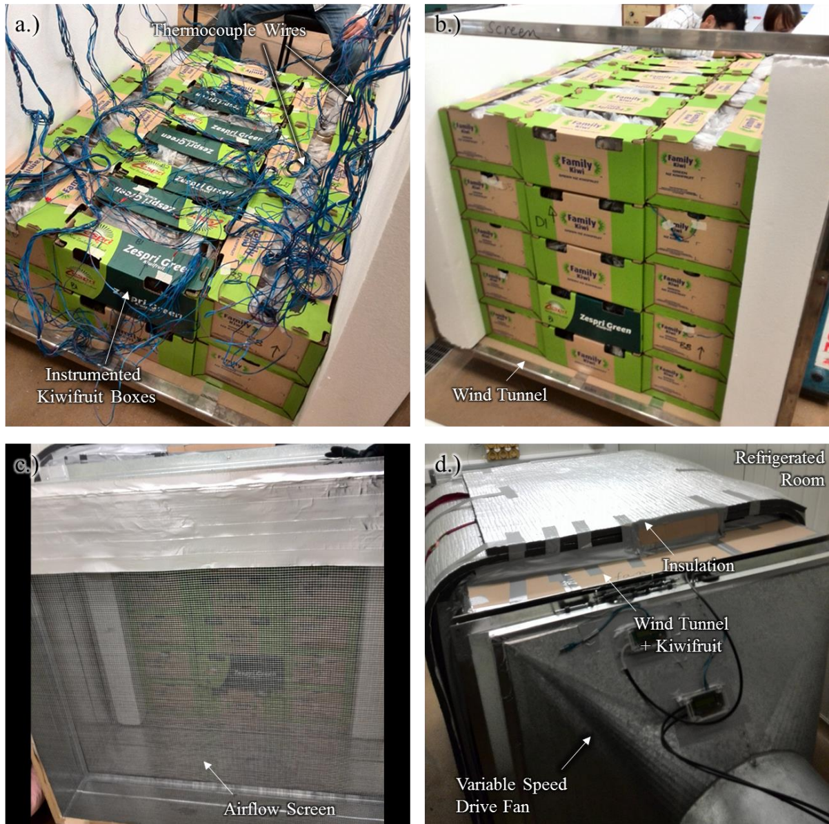
Figure 3.11: Photos of experimental equipment: a.) the wind tunnel with kiwifruit boxes half-way through instrumentation; b.) a fully instrumented wind tunnel; c.) the airflow screen being attached to the wind tunnel; d.) the wind tunnel being attached to the VSD.
