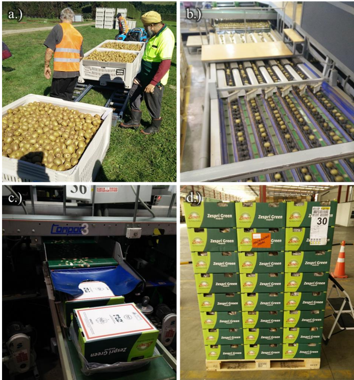
Figure 4.29: The processes involved with filling modular bulk boxes with kiwifruit: a.) fruit are picked and placed into large bins, then delivered by truck to a packing house; b.) fruit are sorted automatically by a grader, which sorts fruit into their various weight categories, including count 36; c.) fruit within the count 36 size range are automatically deposited from the grading line and into a modular bulk box; d.) after boxes are filled, they are stacked into pallets and taken to a forced-air pre-cooler.
