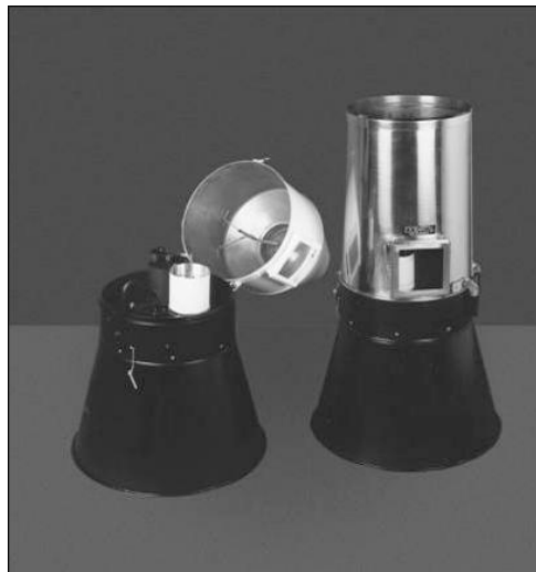
Figure 4.1: A Dines tilting siphon rain gauge. This picture is downloaded from R W Munro Limited web page www.munro-group.co.uk in 2010.
