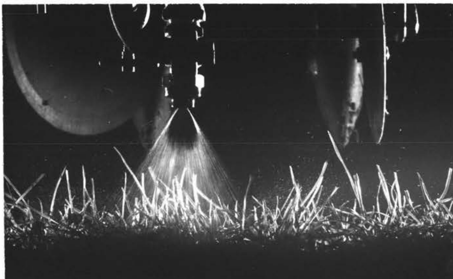
Plate 22. Delevan FS 2.5 Fanjet, 3 in. height, Spraying on to Pasture Surface (head on view).
