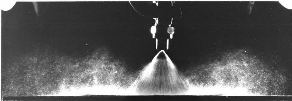
Plate 20. Monarch 6.4 HC Conejet, 1 7/8 in. height, Spraying on to Blotting Paper Surface (head on view).
