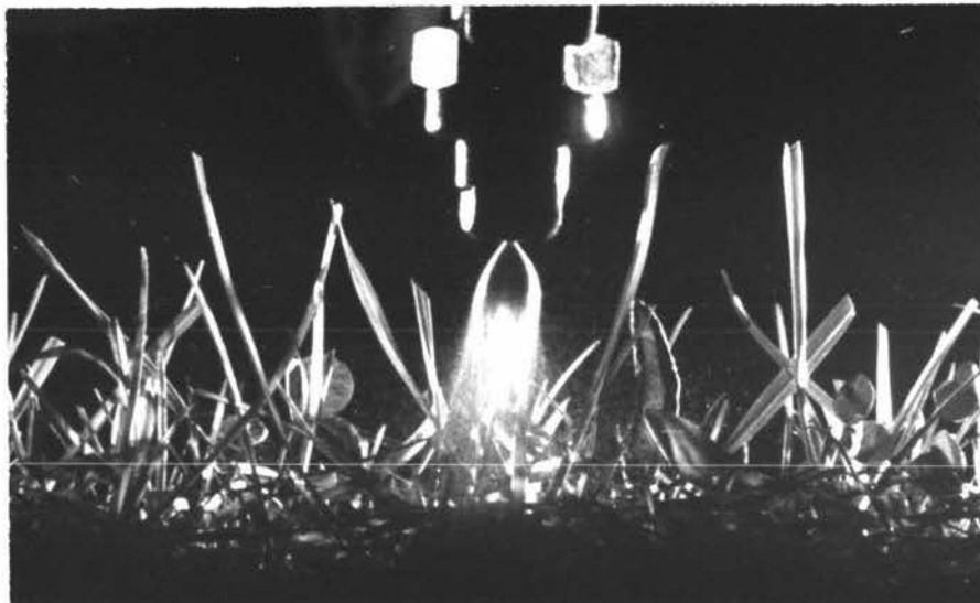
Plate 19. Spraying Systems 4Y 1.5 Conejet, 1-7/16 in. height, Spraying on to Pasture Surface (head on view).
