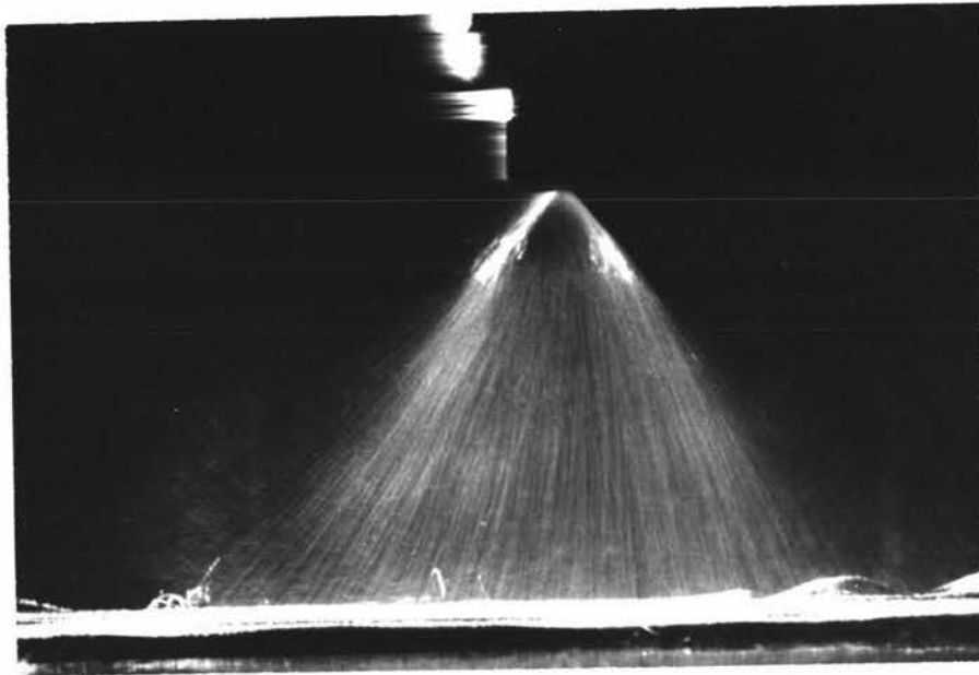
Plate 24. Monarch 6.4 HC Conejet, 1\frac{7}{8} in. height, Spraying on to Felt Surface (side on view).
