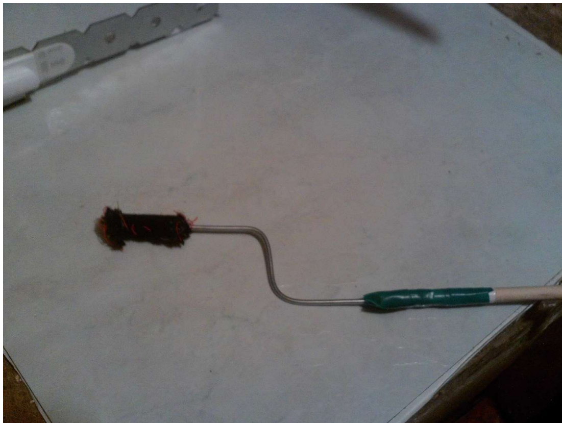
Fig 4. An artificial queen bee attached to the extension fitted to the UAV
