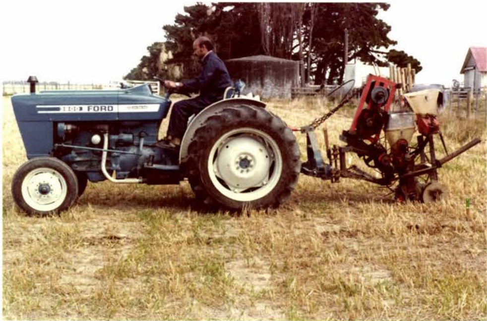
Fig. 10 Test rig and tractor, direct drilling.
