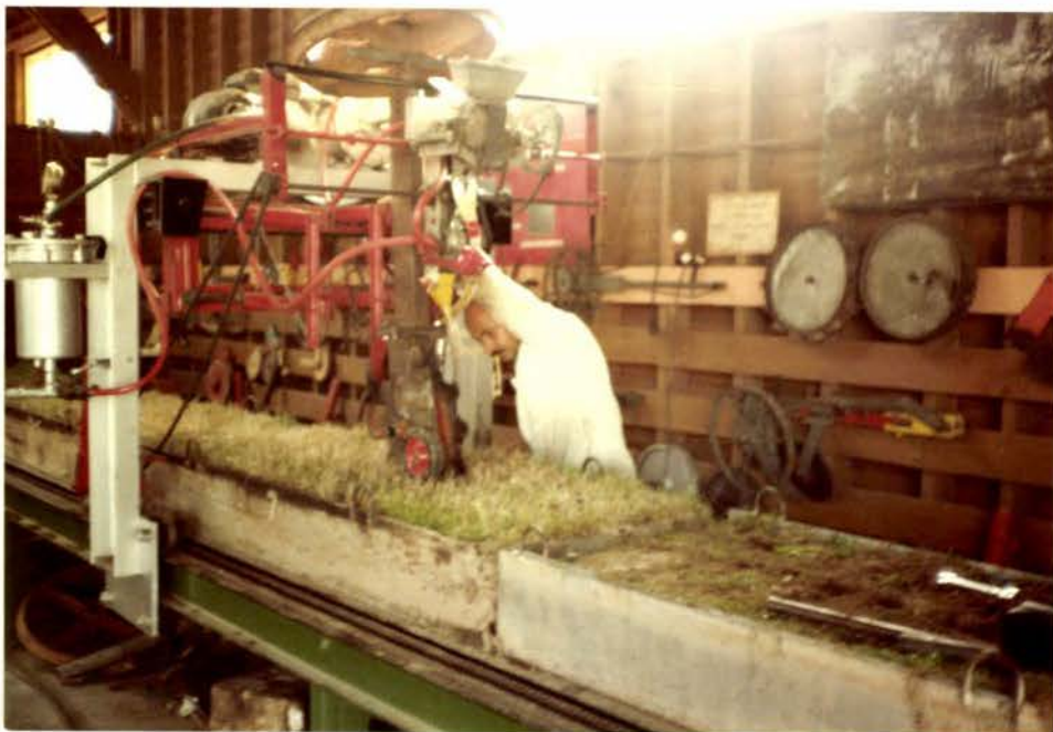
Fig. 23 Direct drilling in progress on the tillage bin, showing gantry and tool testing apparatus.
