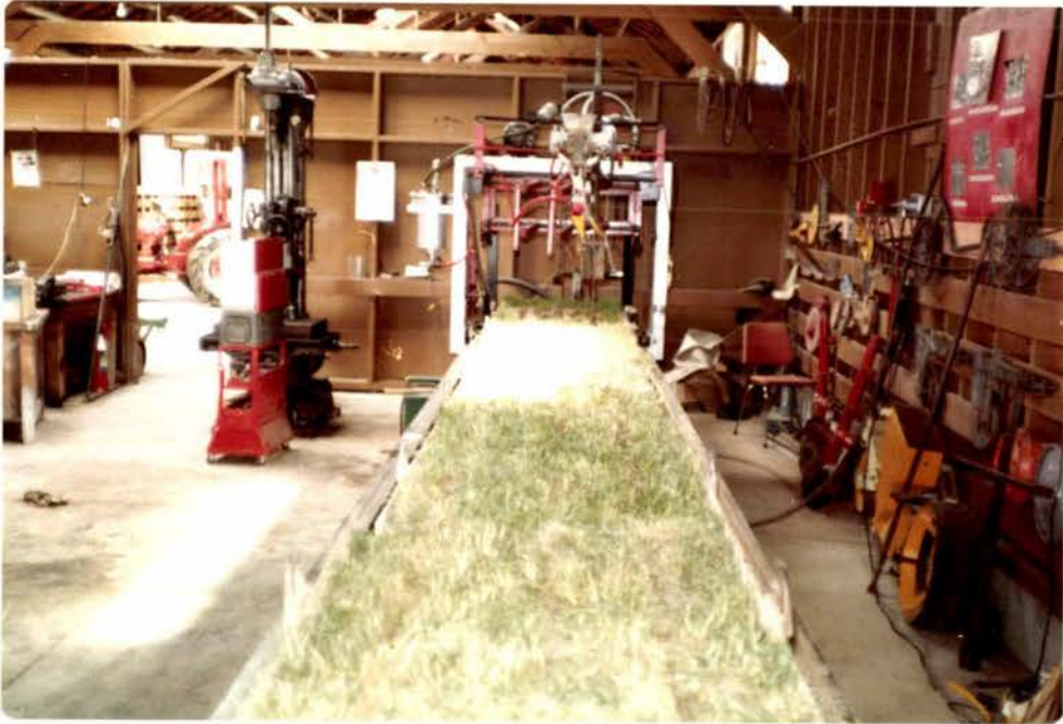
Fig. 24 The turf blocks resting on the support beds after direct drilling (with the gantry at the far end of its travel).
