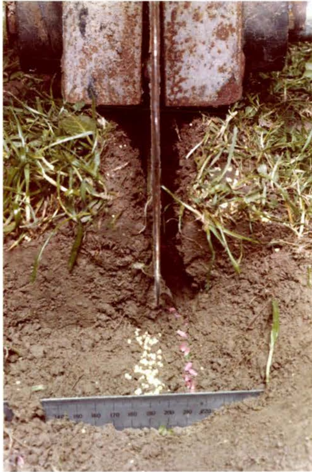
Fig. 11 Chisel coultter and cross section of the groove showing the separate seed and fertiliser distribution.
