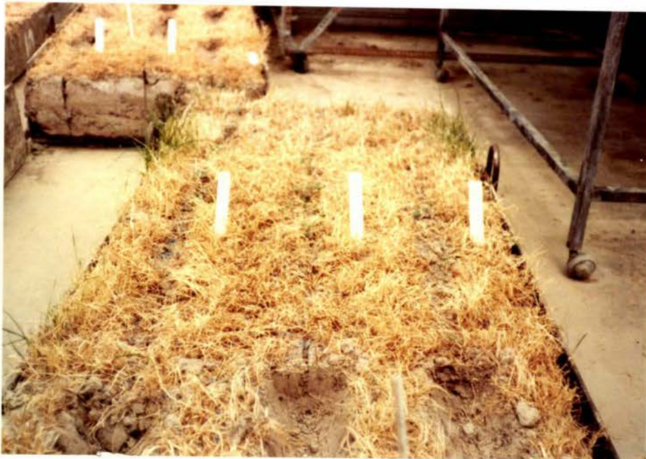
Fig. 33 (Foreground) The divots formed by the scoop sampler in the turf blocks.
