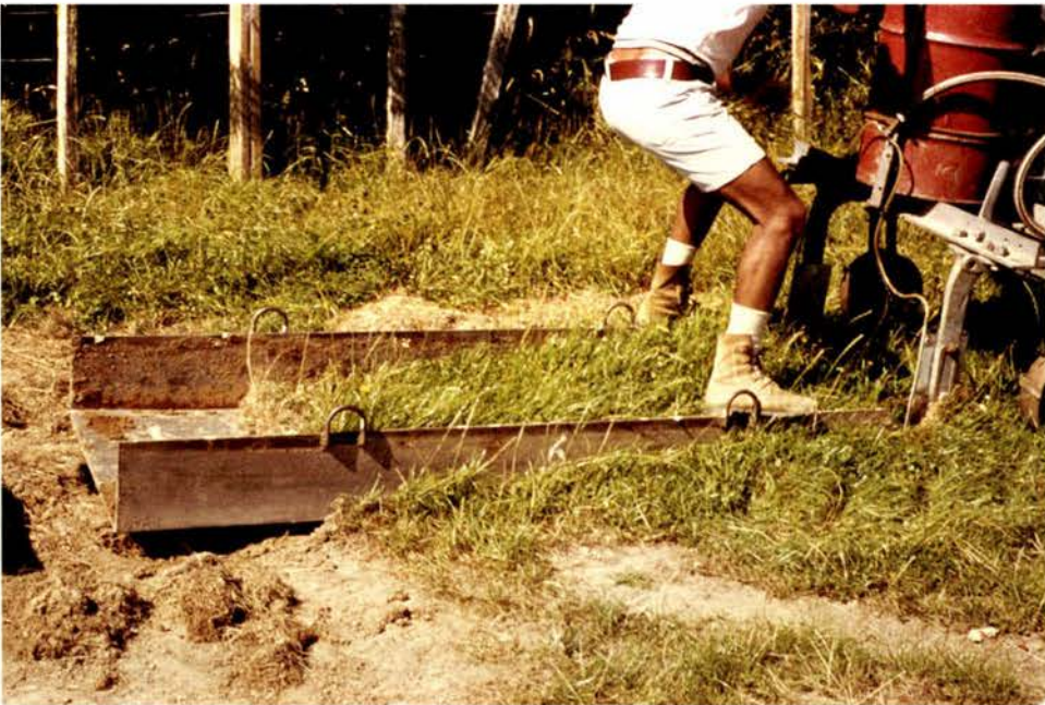
Fig. 15 Bin collection technique; Initial penetration of bin into soil.
