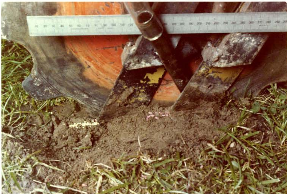
Fig. 31 A side view of vertical placement coulter assembly in the soil after removal of soil to expose wheat seed and fertiliser.
