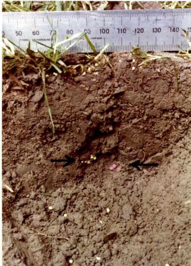
Fig. 8 Cross section of a groove formed with the improved chisel coulter showing seed (right) and fertiliser (left) placement.
