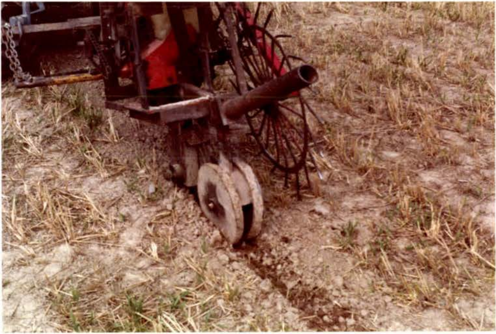
Fig. 9 Rear view of the press wheels and test rig, drilling in a rotary hoed plot.
