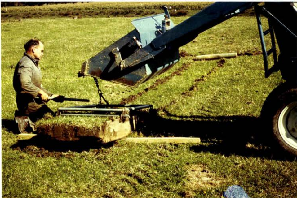
Fig. 17 Bin collection technique; tillage bin removed with a front end loader.
