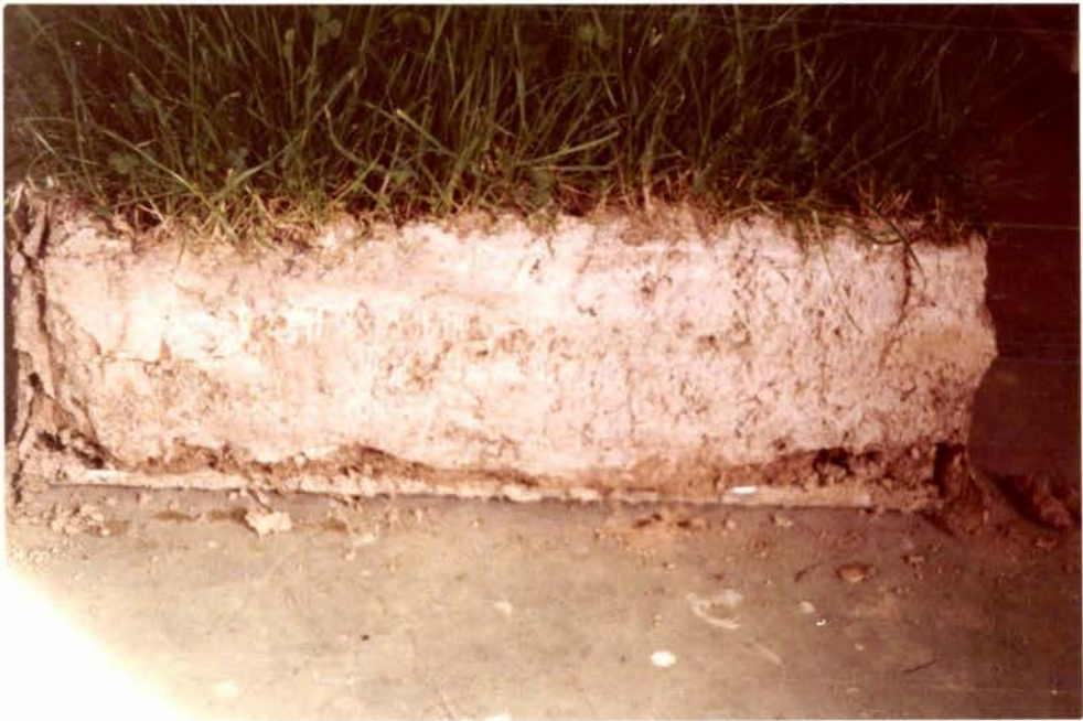
Fig. 20 Open end of a turf block, after coating with paraffin wax.
