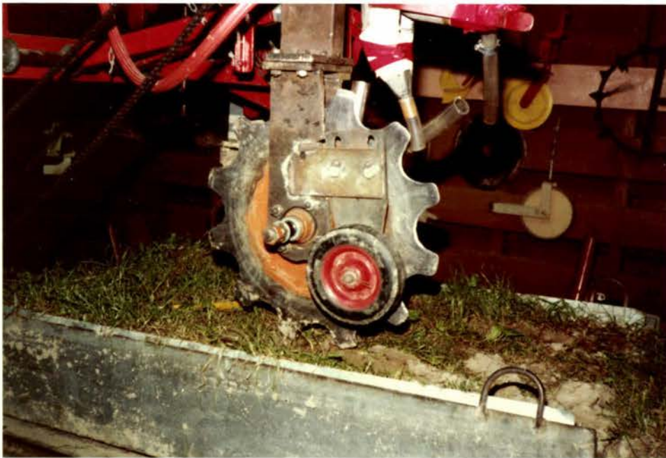
Fig. 29 The depth control wheel attached on the modified improved chisel coulter.
