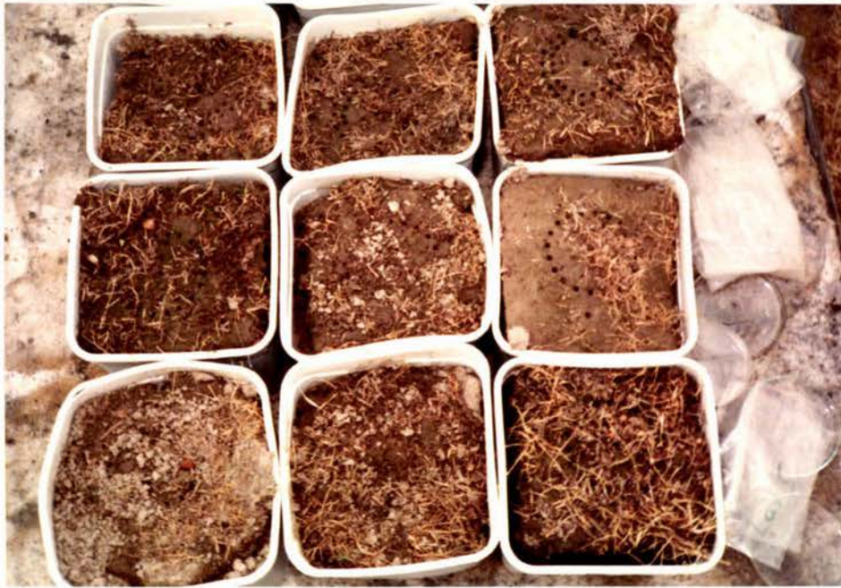
Fig. 4 The filling of "pre-drilled" holes and earthworm activity. Some holes have completely disappeared.
