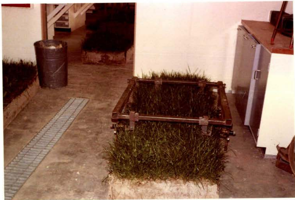
Fig. 19 A specially constructed lowbed wheeled trolley straddling a turf block.
