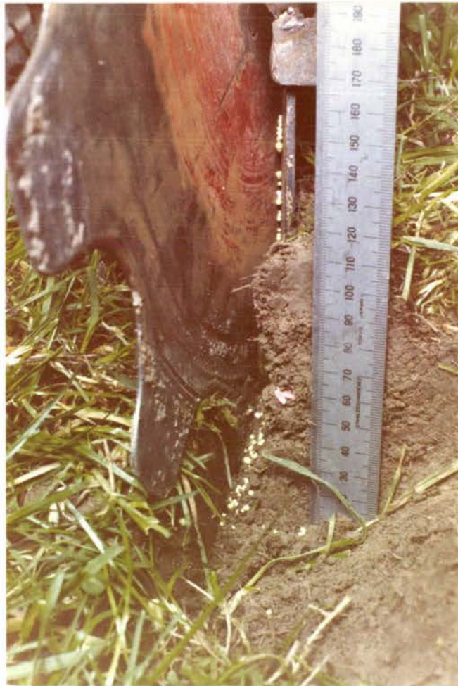
Fig. 30 A cross sectional rear view of modified chisel coulter for vertical placement: Wheat seed (at 60mm level on scale) and fertiliser at 40mm level.
