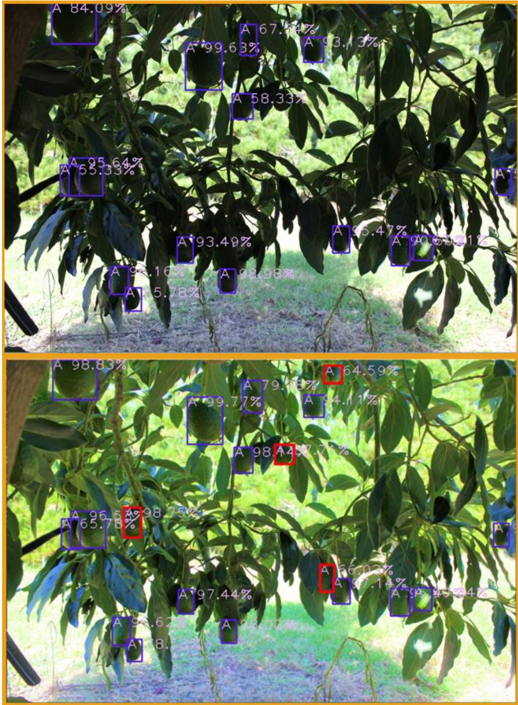
Figure 4.3. (Top) Showing a detection result of the YOLOv3 model on a test photo from the preliminary orchard photo dataset, real detection conditions. (Bottom) A modified version with saturation and brightness increased by 100% respectively. ‘A’ is the label representing avocado, and the percentage value is the confidence level.
